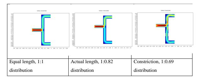
Figure 23: Computational fluid dynamics on the fuel cell air delivery system <sup>50</sup>
