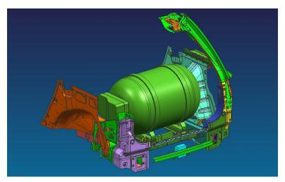
Figure 21: Hydrogen tank location on the Chevrolet Equinox vehicle
