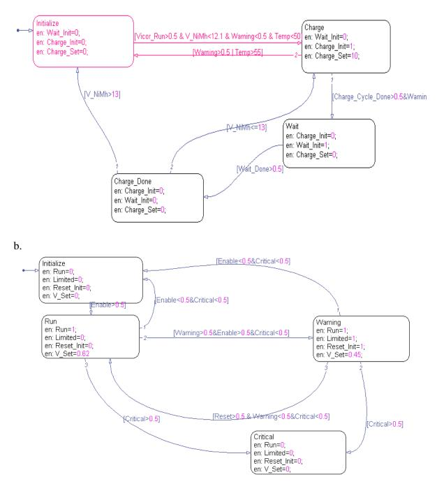
Figure 36: Battery control stateflow (a). Vicor safety stateflow (b)
