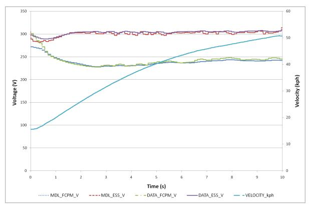
Figure 56: Validation of model predicted bus voltages vs vehicle acceleration data
