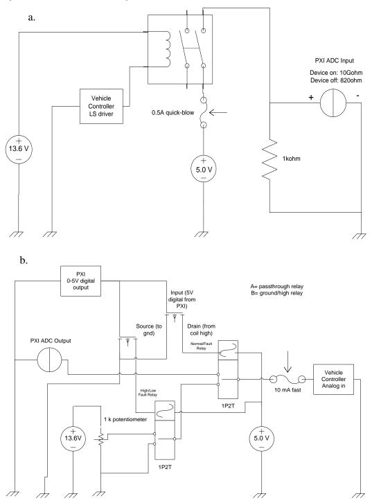
Figure 26: HIL system circuits. Low-side relay driver (a) Failure insertion (b)
