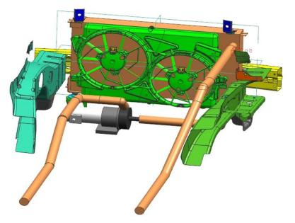
Figure 24: Fuel cell heat rejection system packaging solid model
