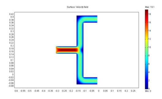
F1: Equal length fuel cell air feed results in 1:1 distribution
