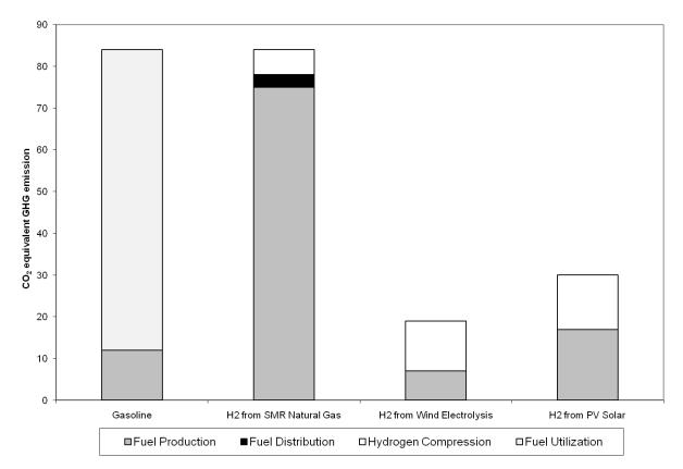
Figure 4: Lifecycle analysis of promising hydrogen production methods <sup>14</sup>
