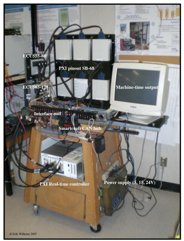
F4: Hardware in the loop simulation system
