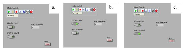
Figure 50: Undesired controller response to 'IGBT ok?' failure. No inserted line failure (a). Inserted short high (b). Inserted short to ground (c)
