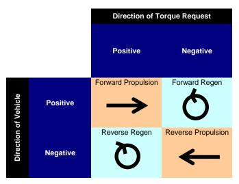
Figure 57: Intended torque control algorithm
