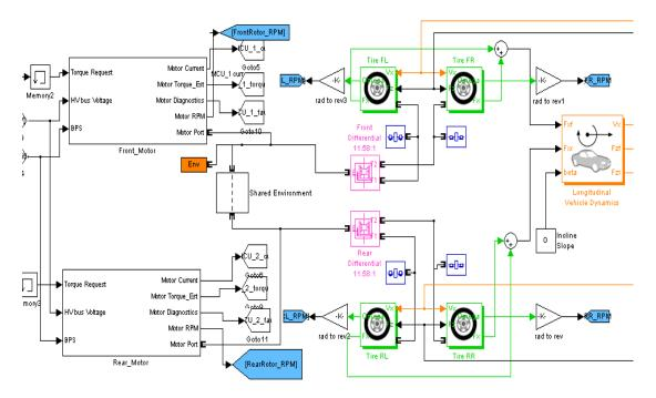
Figure D3: Dynamic plant model – note simdriveline based dynamic performance
