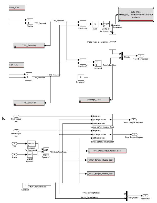
Figure 55: TPS safety variable partial implementation (a). Proposed location for TPS safety variable (b)
