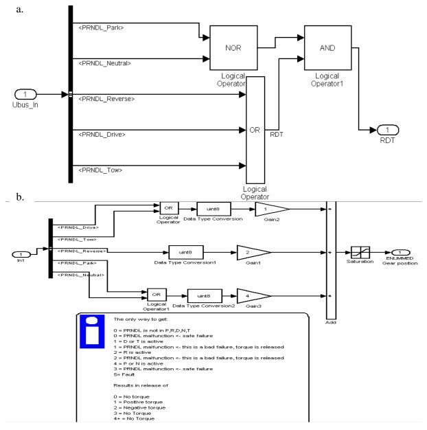
Figure 52: Implemented torque pass-through arbitration (a). Recommended torque pass-through arbitration (b)
