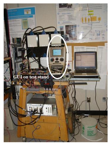
Figure 40: Graphical user interface being developed on the HIL system
