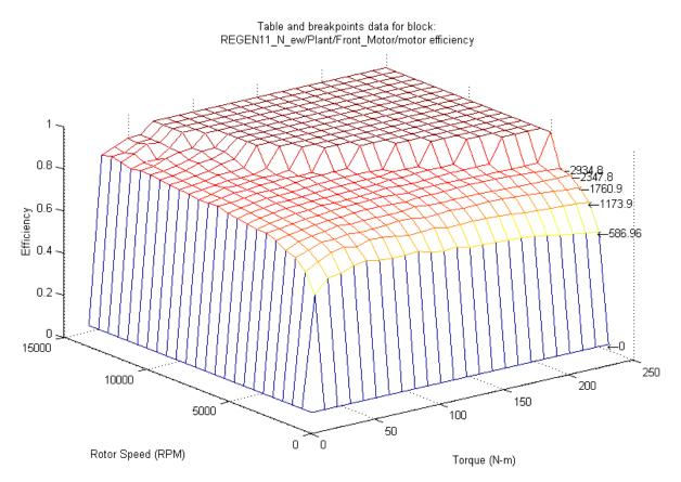
Figure 35: Efficiency table for the Ballard 312V67 MG AC induction motors
