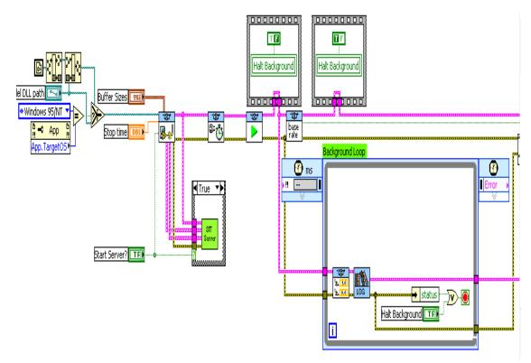
Figure C3: SIT CAN driver VI – note base rate subVI where all IO actions take place
