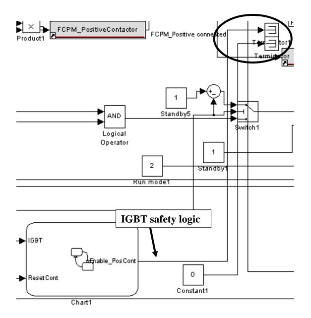
Figure 51: Terminated safety logic in competition controller code
