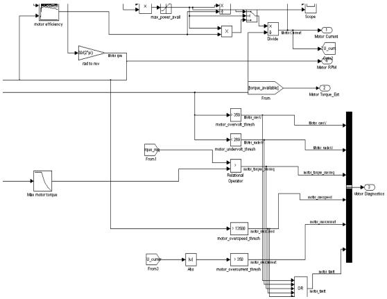
Figure D4: Motor plant model – note motor diagnostics and efficiency/torque inputs
