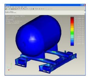
Figure 20: Finite Element Analysis on hydrogen tank mounting structure
