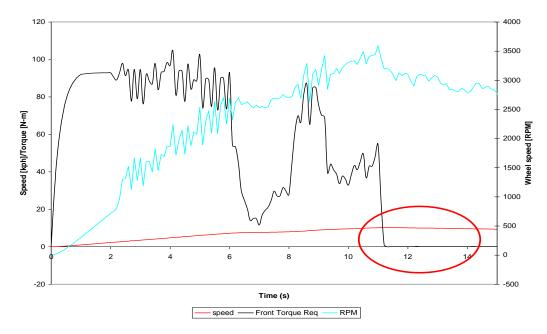
Figure 58: Regenerative braking control strategy not functioning as intended
