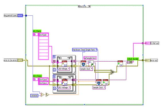
Figure C4: SIT DAQ initialize channel VI – note that even for only performing AO operation AI is defined
