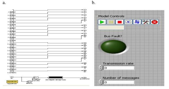
Figure 29: Bus loader model (a) and associated CAN transmission VI for the PXI (b)
