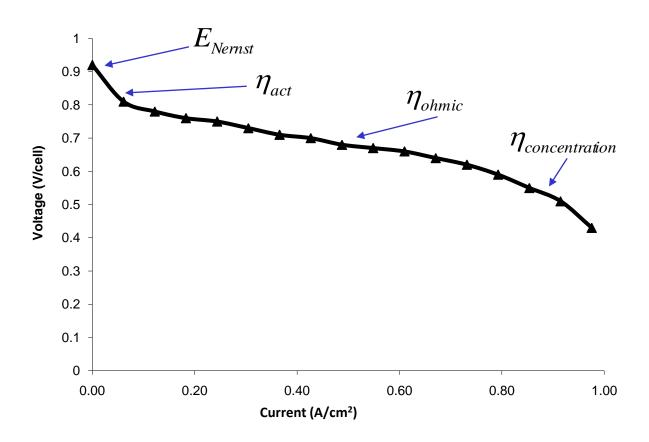
Figure 12: Polarization curve showing the operating characteristics of a fuel cell
