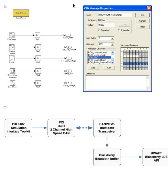
Figure 39: Bluetooth to CAN development on the HIL system. Simple HIL model (a) Battery CAN message definition (b) Data transmission pathway (c)
