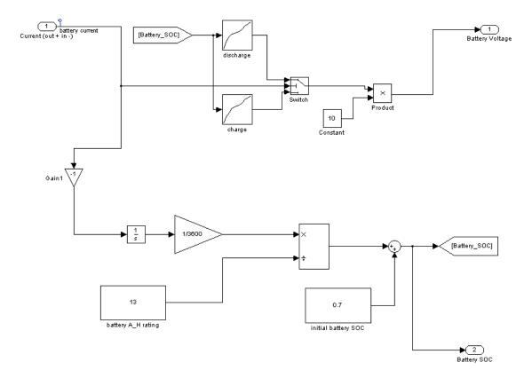
Figure 37: 12V NiMH battery Simulink model
