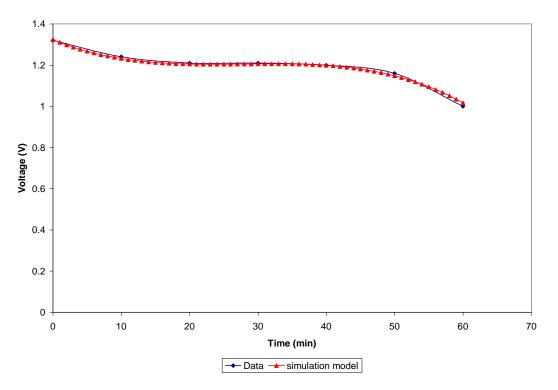
Figure 60: Empirical NiMH battery system model fit
