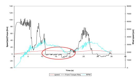
Figure 59: Regenerative braking control strategy functioning as intended
