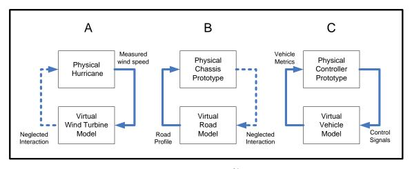
Figure 14: Examples of uni- and bidirectional simulation <sup>26</sup>
