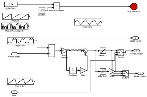
Figure D2: Drive cycle input- speed in m/s into a repeating sequence block. Stop simulation when one sequence has been completed
