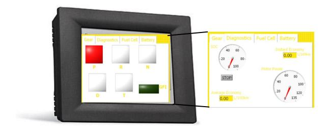
Figure 65: TPC-2006 touch screen with custom UWAFT interface <sup>41</sup>
