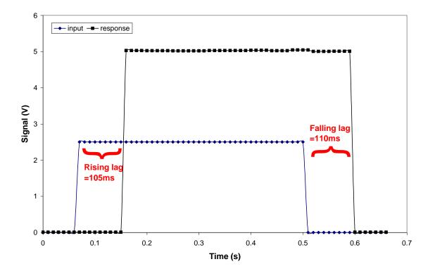
Figure 42: Lag resulting from signal bus test with PXI simulator sleep
