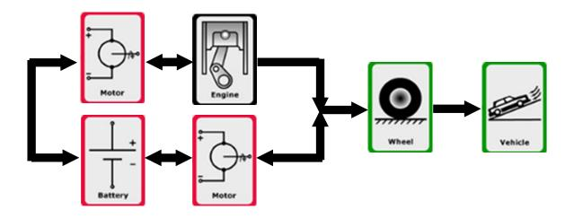
Figure 9: Series-parallel hybrid vehicle configuration <sup>44</sup>
