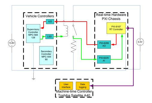
Figure 27: Communication lag test data flow: Begins red, ends green
