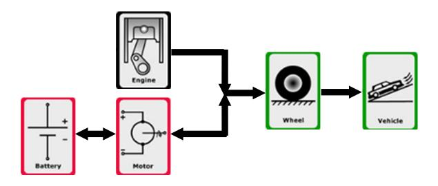
Figure 7: Parallel hybrid vehicle configuration <sup>44</sup>
