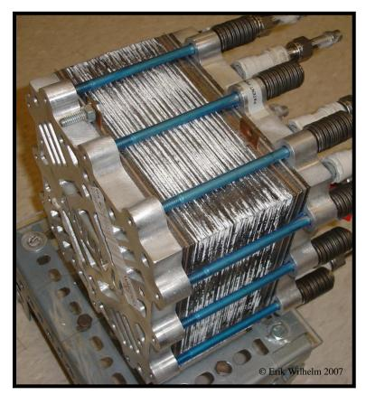
Figure 13: Fuel cell stack comprised of 18 cells in series
