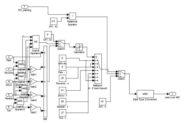
Figure 41: GUI vehicle controller interface code
