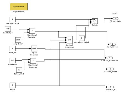
Figure 30: Fuel cell power module fault insertion model
