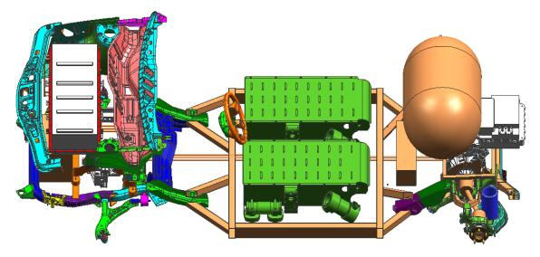
Figure 17: Powertrain packaging for the fuel cell Chevrolet Equinox
