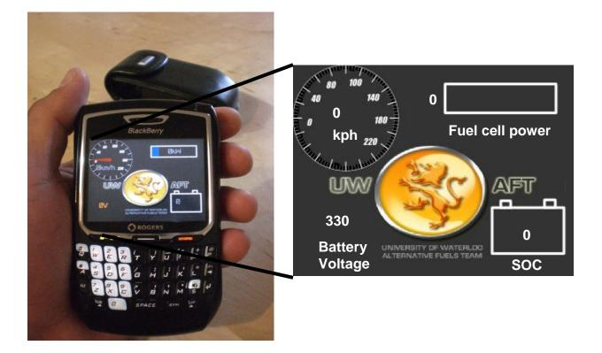
Figure 64: Bluetooth CAN message receiver on the Blackberry<sup>™</sup> device
