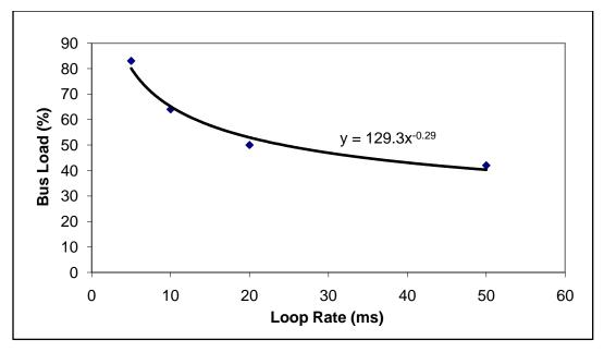
Figure 47: Bus load as a function of 13 message transmission loop rate
