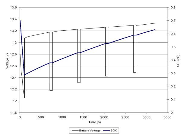
Figure 62: Expected charge circuit function. Charging the battery is interrupted periodically for 1 minute intervals to measure the battery state of charge
