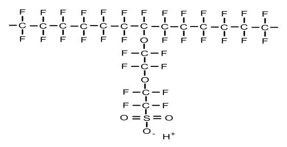
Figure 11: Polymer electrolyte membrane structure: sulphonated flouroethylene
