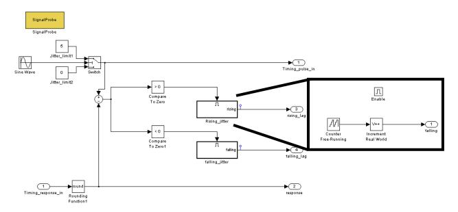
Figure 28: Timing pulse algorithm. Inset: Rising jitter triggered subsystem
