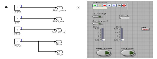
Figure 33: Failure insertion plant model. Simulink model (a) Labview control (b)
