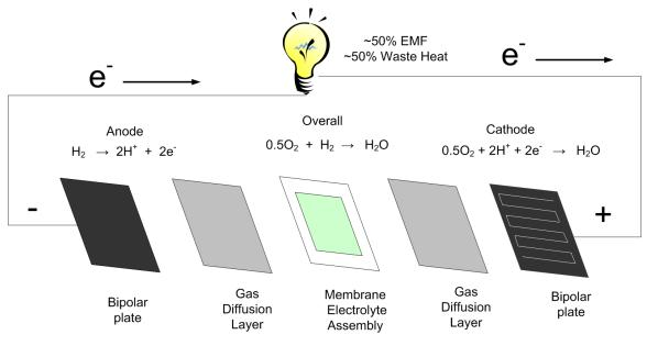
Figure 10: Single polymer electrolyte fuel cell
