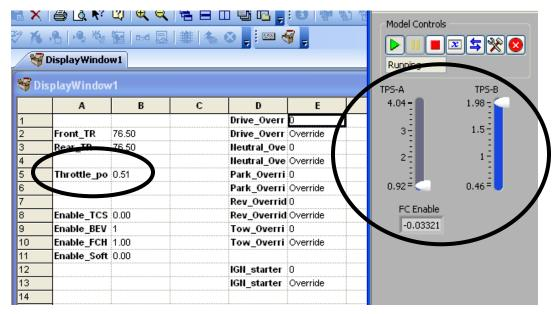
Figure 53: Averaged instead of zeroed throttle position value when sensors disagree
