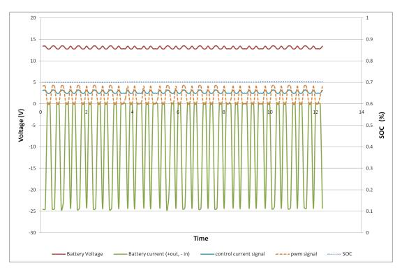
and low charge current requests from the controller. Oscilloscope probing ruled out the possibility of signal transmission error.
