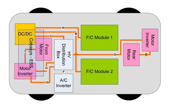
Figure 18: Major wiring conduits on the fuel cell Equinox
