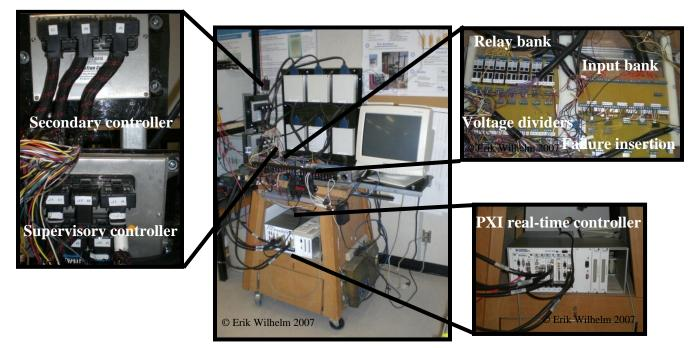
Figure 25: A Hardware-in-the-loop simulation system for a fuel cell Chevy Equinox
