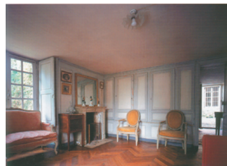
3-36, 3-37, 3-38 The low ceiling of a small cabinet conceals an entresol floor above, connected by a hidden stair.
