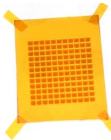
Figure 4.6: Kapton substrate held in place on a metal chuck for vacuum metal deposition.
