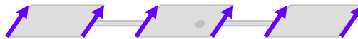
Figure 3.6: Equivalent magnetic line sources showing even-mode coupling between centre and parasitic patch antennas.
