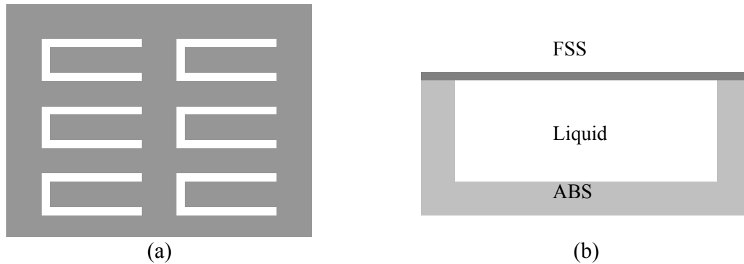
Figure 2.11: Tunable FSS from [35]. (a) Top view showing 6.5mm wide unit cells with 0.3mm wide slots (b) cross-sectional view showing 2mm thick liquid-filled cavity behind the FSS
