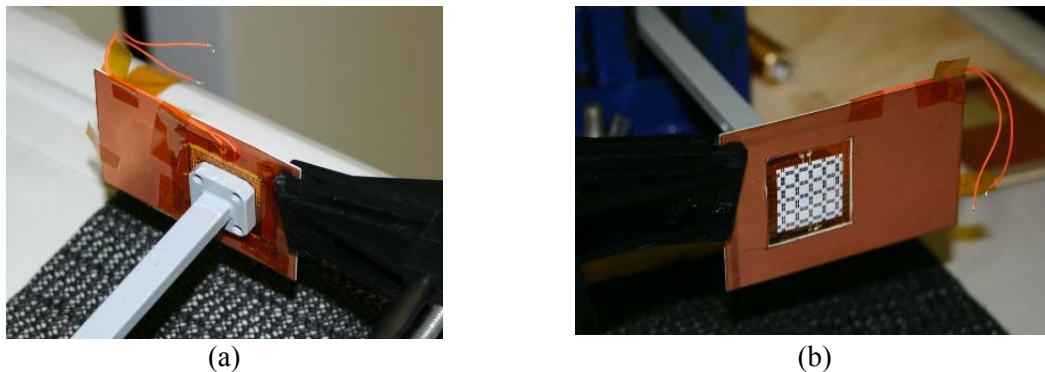
Figure 5.17: Test set used to measure FSS. (a) View from back. (b) View from Front.
