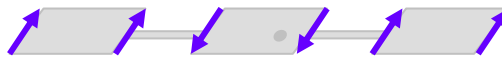
Figure 3.5: Equivalent magnetic line sources showing odd-mode coupling between centre and parasitic patch antennas.
