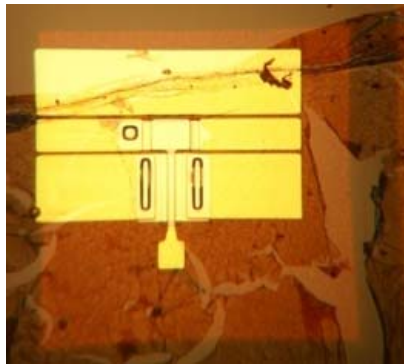
Figure 4.17: Hardened AZ3330 remaining on MEMS device after unsuccessful release.
