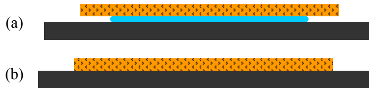
Figure 4.3: Flexible substrate held to rigid wafer by (a) placing a small drop of DI water between the substrate and carrier and (b) heating substrate such that the surface tension pulls the substrates together as the water evaporates.
