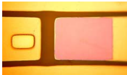
Figure 4.16: Partially fabricated MEMS device showing titanium adhesion layer under silicon dioxide dielectric region.
