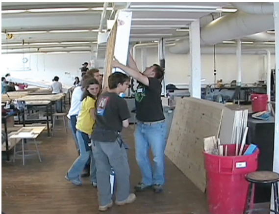
Above Left: 2.89 Lifting a wall panel off its jig.
