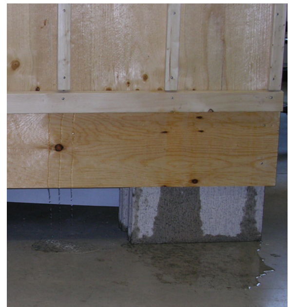
Below: 2.25 A successful water test.
