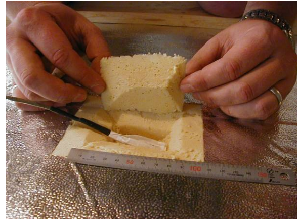
Figure 5.27: Installation of temperature/RH sensor in foam board (Wall 3)
