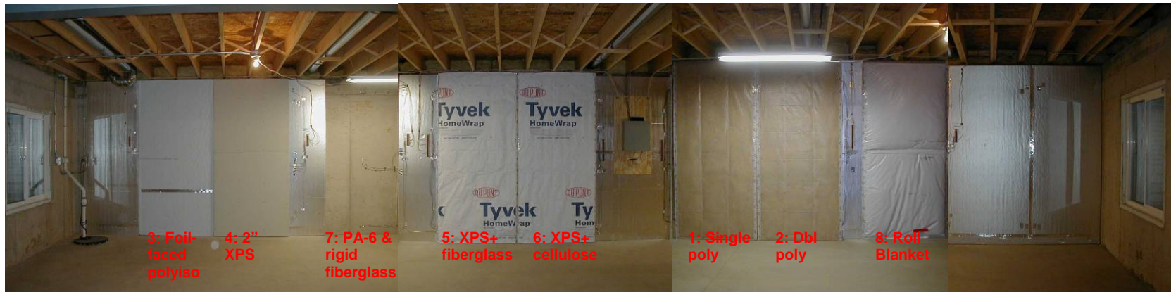
Figure 5.39: Composite photo of test panels in Huntley (prior to wall 7 installation)
