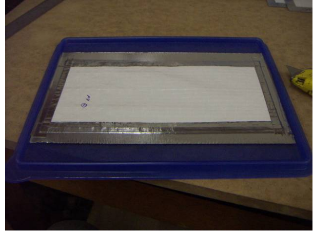
Figure 38: Sample sealed to container lid with foil tape
