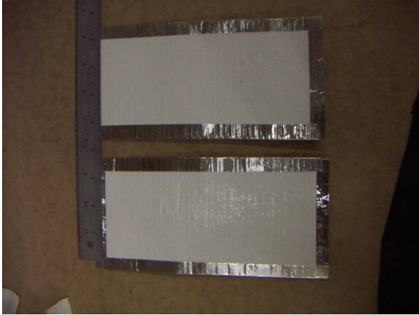
Figure 37: Sample edges wrapped with foil tape
