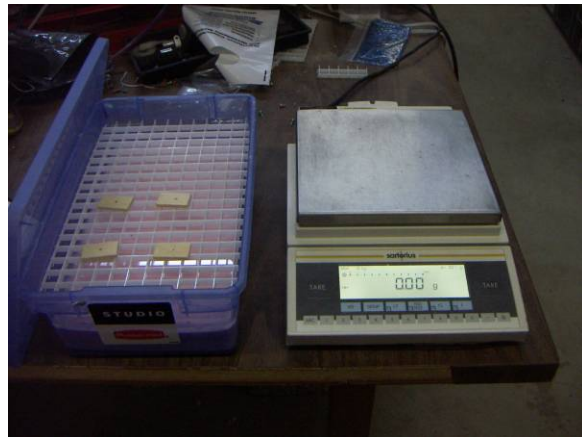
Figure 14: Wafer stock in 100% humidity calibration enclosure with balance
