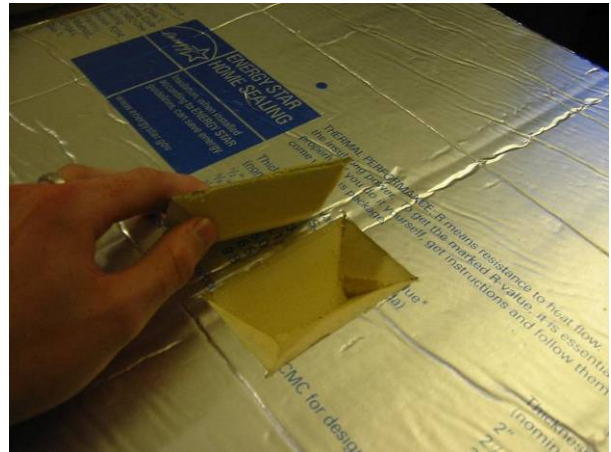
Figure 45: View of access port cut into center of each specimen
