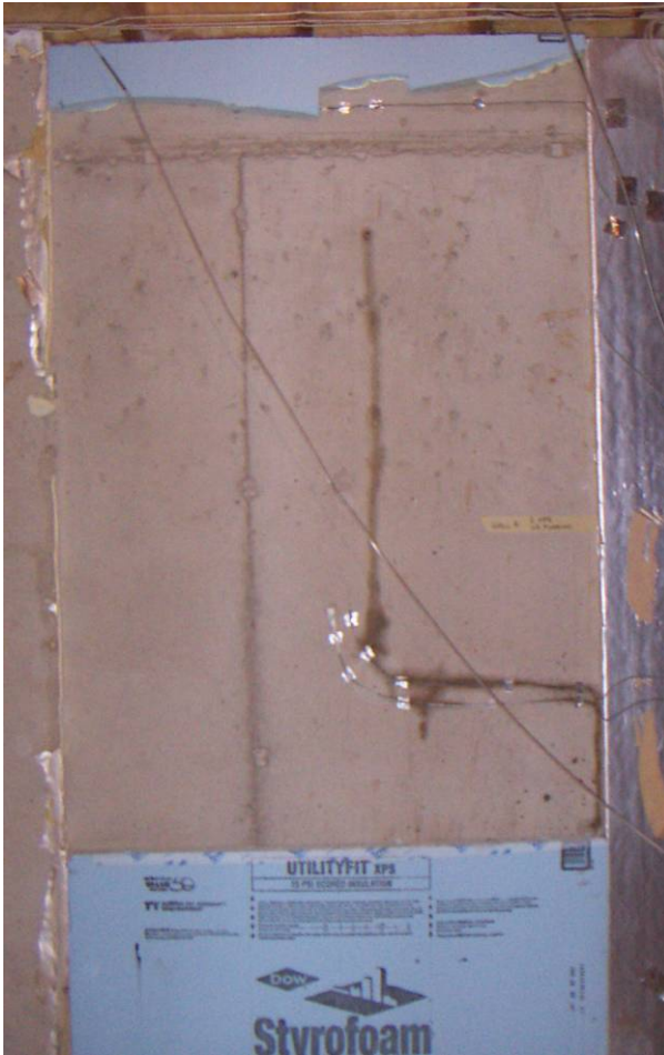
Figure 6.69: Wetting plume in 2" XPS wall
