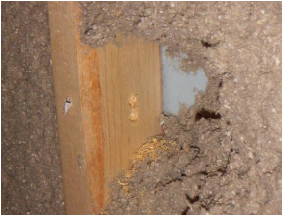
Figure 55: Holes drilled into test stud for sub-surface MC measurements
