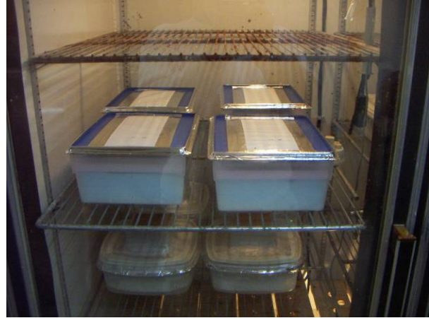
Figure 40: Testing at elevated humidity levels in environmental chamber
