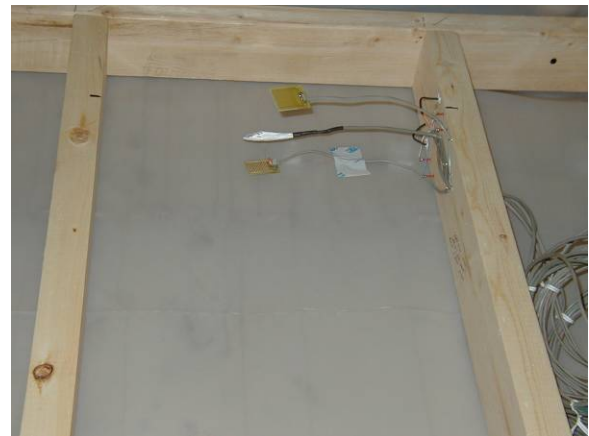
Figure 5.25: Instrumentation package at upper location of stud frame walls (Wall 2)
