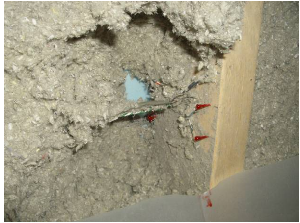
Figure 52: MC pin painting with non-conductive coating, 10/04
