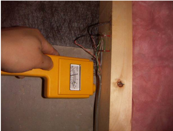
Figure 7.38: Moisture meter measurements of the test bay stud, parallel to MC pins
