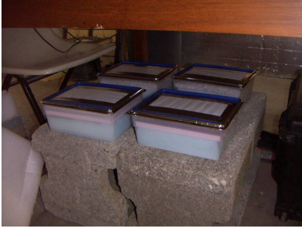
Figure 39: Testing at 20° C/50% RH in climate-controlled test laboratory
