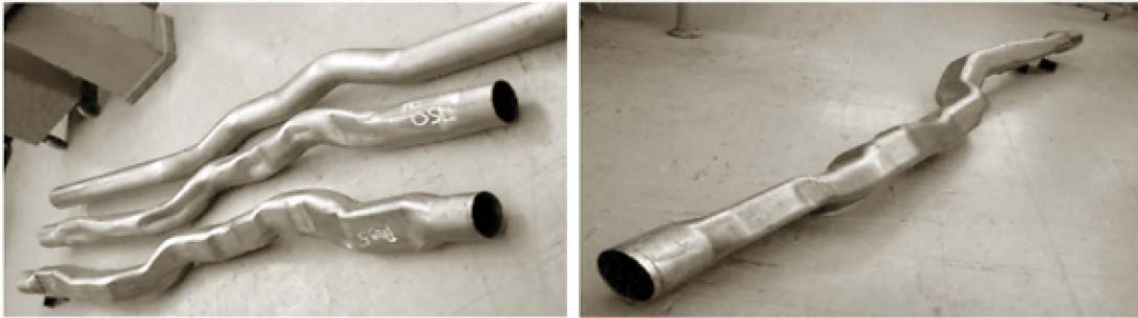
Figure 11: Typical pre-bent, crushed and hydroformed part [1]
