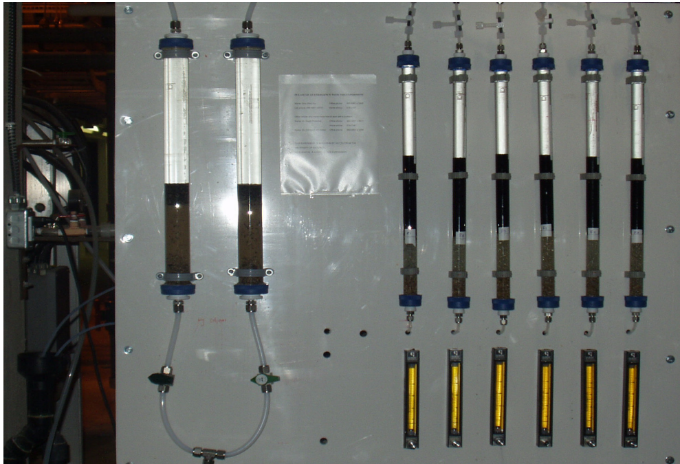
Figure 5-3 GAC preloading facilities
