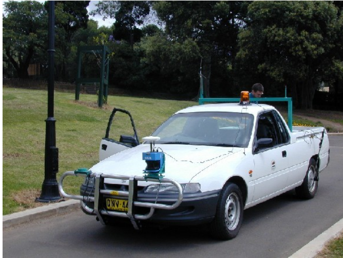
Figure 4.2: Data gathering vehicle. Note the location of the GPS antenna and laser scanner on the front bumper of the truck and the rotary encoder on the rear left wheel.
