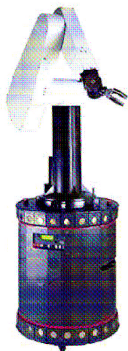
Figure 1.22: Nomadic XR4000 platform with PUMA 560 manipulator [16].
