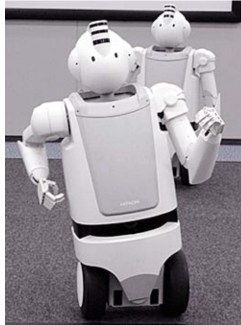
Figure 1.24: Hitachi’s dynamic balancing two-wheeled robot with side-ways tilt joint [60].
