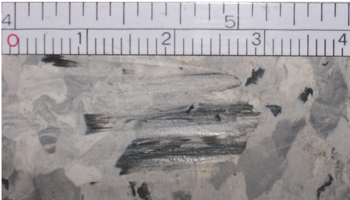
Figure 5.7: Top view of skid marks and slight damage of floor under heaviest load; note large width of indentation and low depth due to wider contact area. Lower ruler scale in cm.
