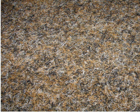
Figure 5.10: Close-up of short-pile commercial carpet test surface.
