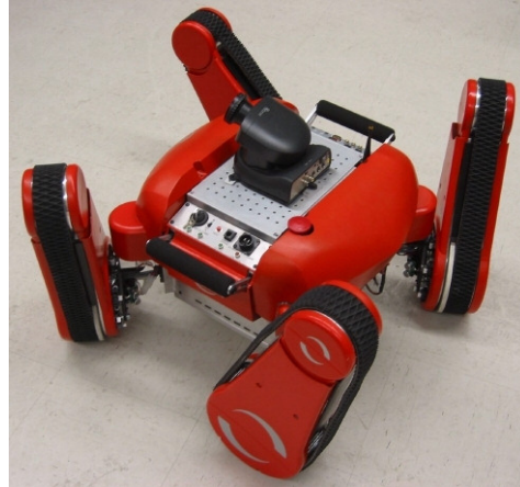
Figure 1.20: Azimut tracked robot [50]
