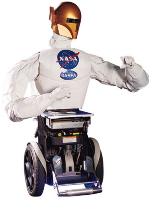
Figure 1.23: The NASA Robonaut mounted on the Segway RMP with custom ‘training wheels’ [55].
