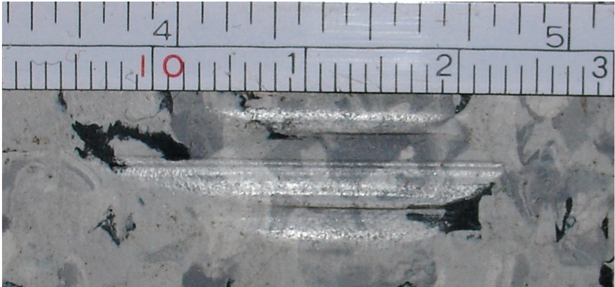
Figure 5.9: Top view of indentation of floor under lightest load; note narrow width of indentation and high depth due to wider contact area. Lower ruler scale in cm.
