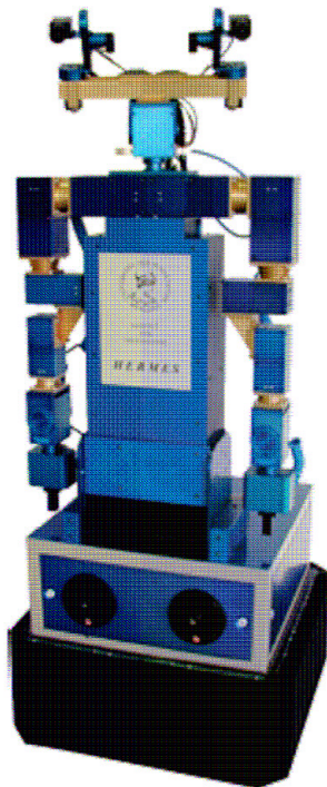
Figure 1.21: HERMES, a statically stable humanoid [51].
