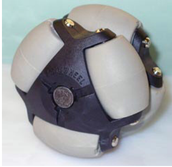
Figure 1.7: A pair of Omniwheel universal wheels from Kornylak Corporation [27].
