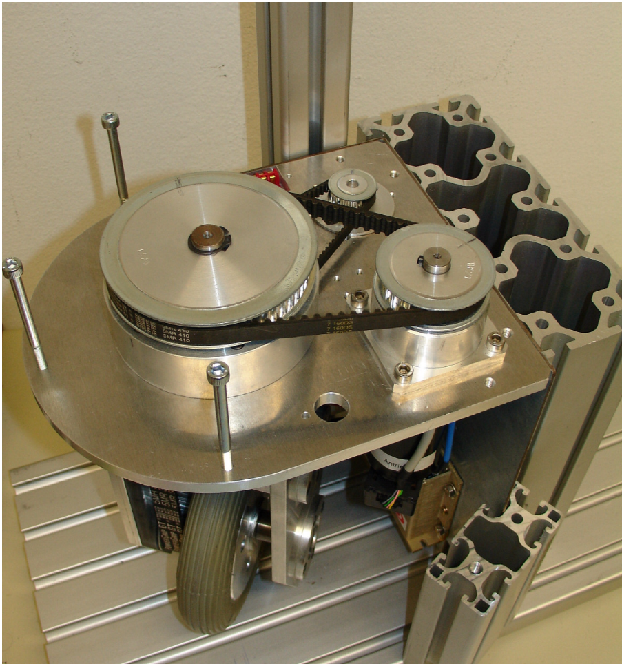
Figure 5.4: test stand with drive unit.
