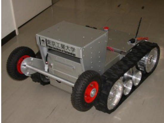
Figure 1.19: HELIOUS-VI tracked robot [49]
