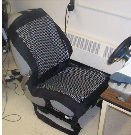
Figure 3.6: Depiction of the experimental driver's seat outfitted with two 36 X 36 pressure mapping pads.
