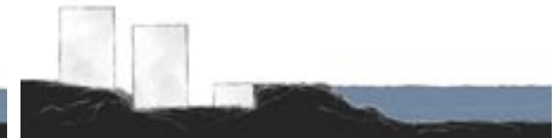
21 New Flood Berm: to be constructed so that all settlements will be protected during flood.
