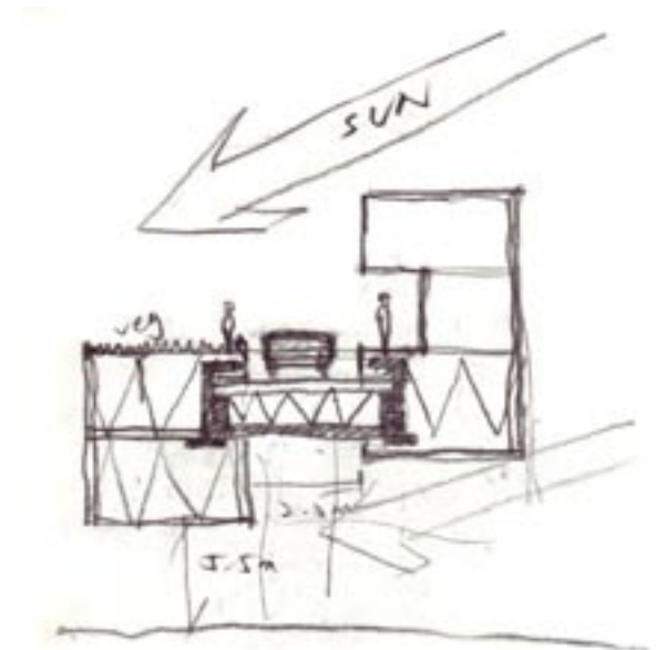
06 Land Over Water Preliminary Section: First attempt at the Land Over Water system in section. The buildings are designed to clip onto the central platform.
