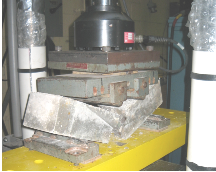
Figure 4.6 Prism after failure under four-point bending conditions.
