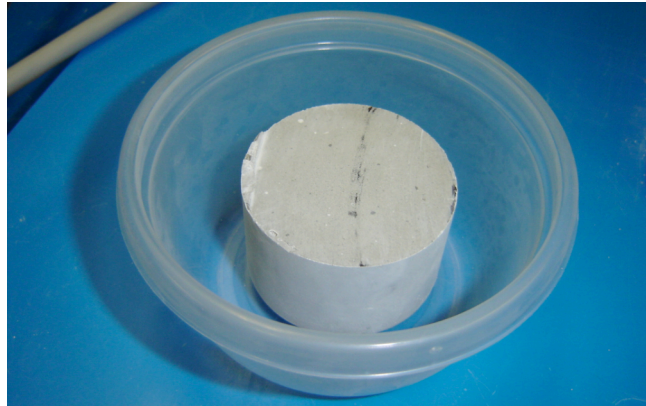
Figure 3.2. Setup of a 50mm \varnothing x 200 mm cement paste specimen in a container for the submersion test.
