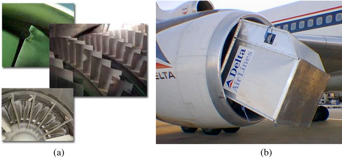
Figure 1.1 (a) Jet engine turbine blade damages [FODNews]; (b) Example of a cargo box being a large FOD hazard [Unusual Aviation Pictures].
