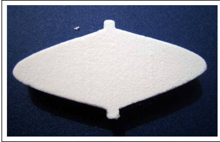
Figure 3-25: Sample of 3DP-fabricated parts showing the surface finish.
