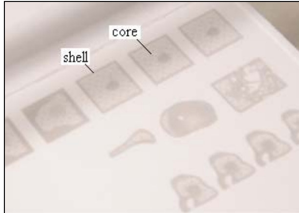
Figure 3-5: Definition of shell and core.
