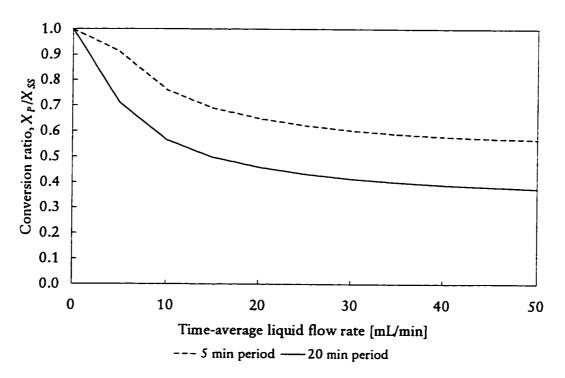
Figure 4.30 Conversion ratios for periodic to steady operation, 0.1 split, 0 - 50 mL/min, 50°C, 1.1 MPa
