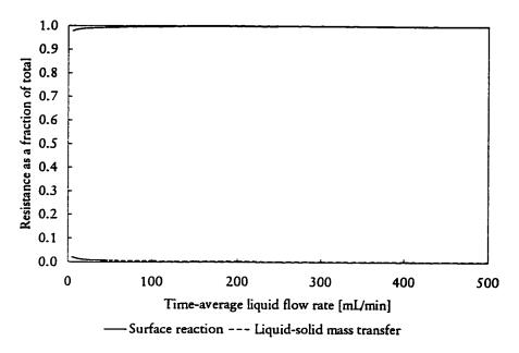
Figure 4.6 Contributing resistances to overall reaction rate as a function of liquid flow rate for steady operation experiments at 50 °C, 0.1 MPa
