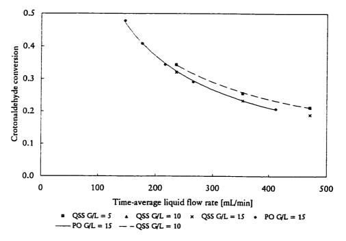
Figure 6.6 Comparison of quasi-steady and periodic operation crotonaldehyde conversion - effect of cycle period
