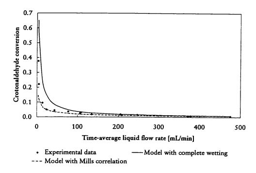
Figure 7.4 Steady operation Model B assuming variable catalyst external wetting with experimental data (Mills-Dudukovic wetting correlation used) and complete catalyst wetting (f = 1)
