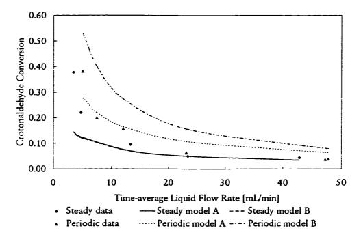
Figure 7.11 Comparison of periodic and steady operation model with experimental data at 25 °C and 1.1 MPa; periodic operation parameters: 0.1 split 20 minute period
