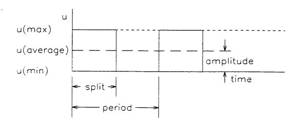
Figure 2.5 Typical square wave used in periodic operation
