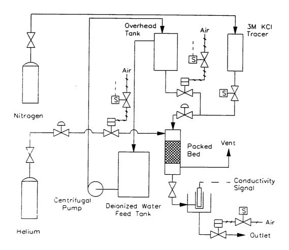
Figure 3.10 Hydrodynamic packed bed flow diagram (S = solenoid actuated valve)
