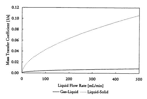
Figure 2.2 Response of mass transfer coefficients (Goto and Smith, 1975a) to liquid flow rate
