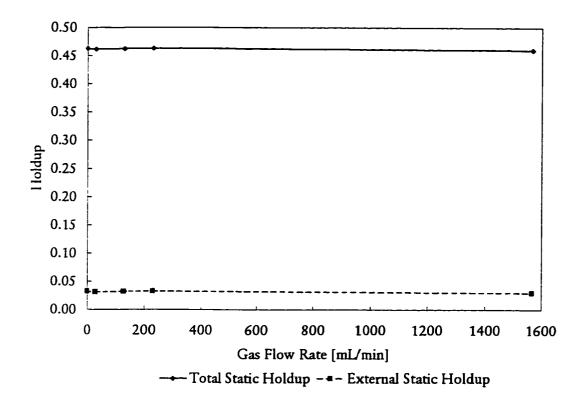
Figure 5.1 Total static liquid holdup and external static liquid holdup as a function of gas flow rate
