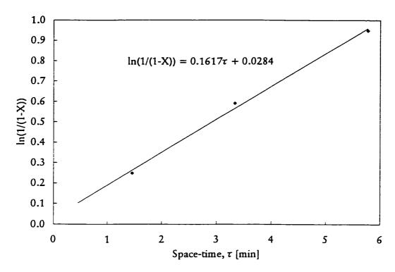
Figure 4.3 First order plot of steady-state data at high liquid flow rates (greater than 100 mL/min) for 50°C and 1.1 MPa
