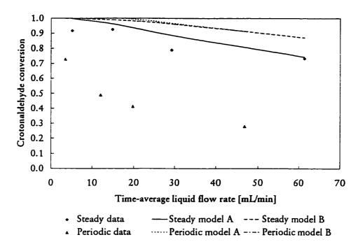
Figure 7.19 Comparison of periodic and steady operation model with experimental data at 50°C and 1.1 MPa; periodic operation parameters: 0.1 split 20 minute period
