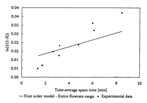
Figure 4.11 First order rate law plot for steady operation, 25 °C, 1.1 MPa Comparison of experimental data, liquid flow rate range: 50 - 450 mL/min with first order model fitted over entire flow rate range (5 - 450 mL/min)
