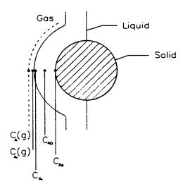
Figure 7.2 Gas-liquid-solid contact at the particle level for Model B
