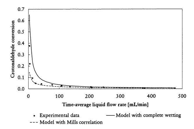
Figure 7.3 Steady operation Model A assuming variable catalyst external wetting with experimental data (Mills-Dudukovic wetting correlation used) and complete catalyst wetting (f = 1)
