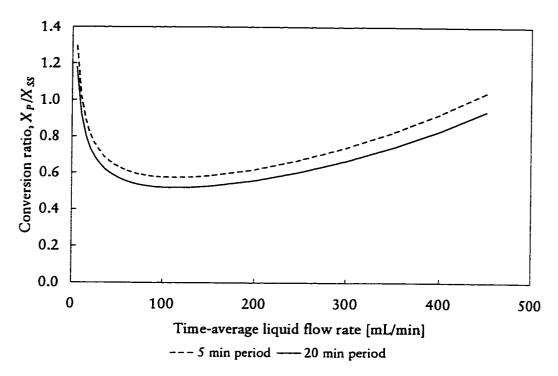
Figure 4.31 Conversion ratios for periodic to steady operation, 0.5 split, 0 - 450 mL/min, 50°C, 1.1 MPa
