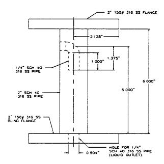
Figure 3.7 Outlet section rotated 90°
