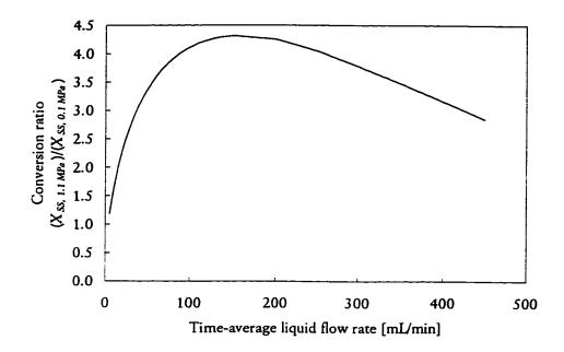
Figure 4.33 Conversion ratio ( $X_{SS, 1.1 \text{ MPa}}/X_{SS, 0.1 \text{ MPa}}$ ) for steady operation at 50°C, 1.1 MPa and 50°C, 0.1 MPa
