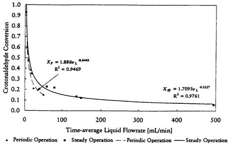
Figure 4.38 Steady and periodic operation (20 min period, 0.1 split) crotonaldehyde conversion vs. liquid flow rate, 50°C, 0.1 MPa
