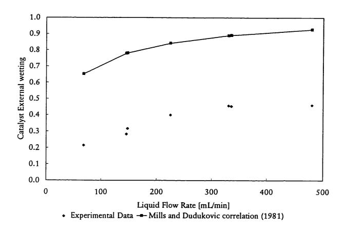
Figure 5.4 Catalyst external wetting efficiency as a function of liquid flow rate
