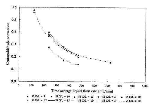
Figure 6.4 Comparison of steady and periodic operation crotonaldehyde conversion - effect of flush duration
