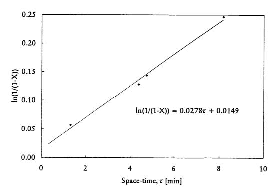
Figure 4.5 First order plot of steady-state data at high liquid flow rates (greater than 100 mL/min) for 50°C and 0.1 MPa
