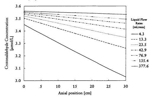
Figure 7.8 Crotonaldehyde concentrations at the catalyst outer surface as predicted by simulation Model A under steady operation at 25°C and 1.1 MPa
