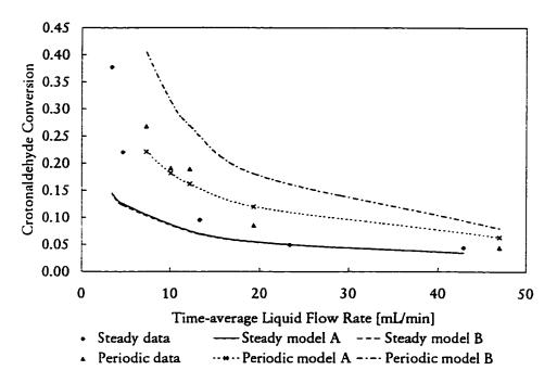
Figure 7.9 Comparison of periodic and steady operation model with experimental data at 25°C and 1.1 MPa; periodic operation parameters: 0.1 split 5 minute period
