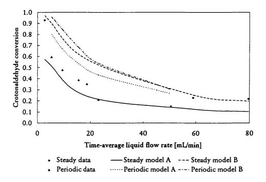
Figure 7.25 Comparison of periodic and steady operation model with experimental data at 50°C and 0.1 MPa; periodic operation parameters: 0.1 split 20 minute period
