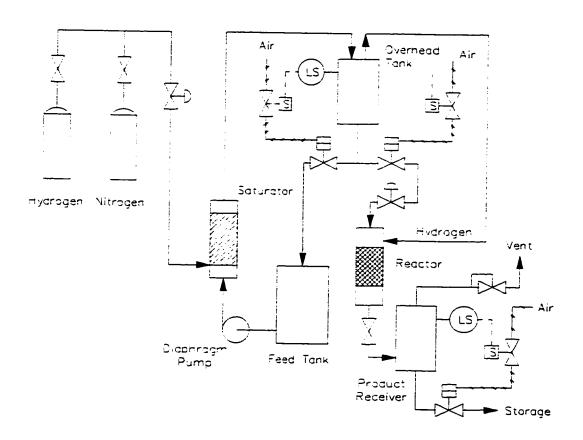
Figure 3.1 Experimental trickle-bed reactor process flow diagram
