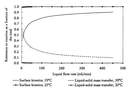
Figure 4.8 Contributing resistances to overall reaction rate as a function of liquid flow rate for steady operation at 25°C and 50 °C, 1.1 MPa, assuming a liquid-solid mass transfer coefficient half that predicted by the Goto-Smith correlation
