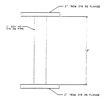
Figure 3.5 Prepacking section
