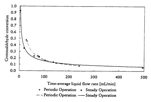
Figure 4.35 Steady and periodic operation (5 min period, 0.5 split) crotonaldehyde conversion vs. liquid flow rate, 50°C, 0.1 MPa
