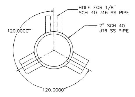
Figure 3.8 Catalyst bed cross-section
