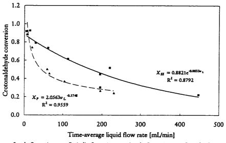
Figure 4.27 Steady and periodic operation 5 min period, 0.5 split Crotonaldehyde conversion vs. liquid flow rate, 50°C, 1.1 MPa
