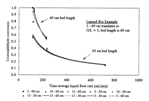
Figure 6.1 Crotonaldehyde conversion as a function of liquid flow rate, gas flow rate and bed depth
