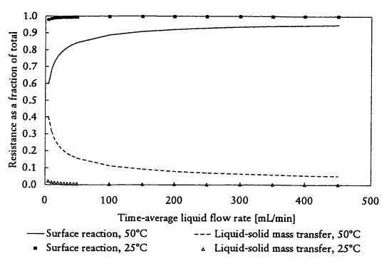
Figure 4.1 Contributing resistances to overall reaction rate as a function of liquid flow rate for steady operation experiments at 25 °C, 1.1 MPa and 50 °C, 1.1 MPa
