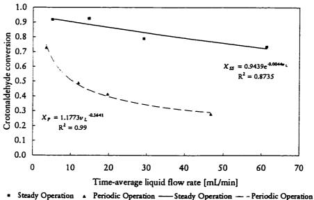
Figure 4.28 Steady and periodic operation 20 min period, 0.1 split Crotonaldehyde conversion vs. liquid flow rate, 50°C, 1.1 MPa
