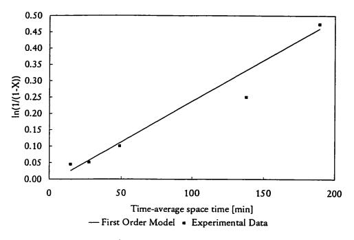
Figure 4.12 Steady operation first order plug flow model 25 °C, 1.1 MPa, liquid flow rate range: 0 - 50 mL/min
