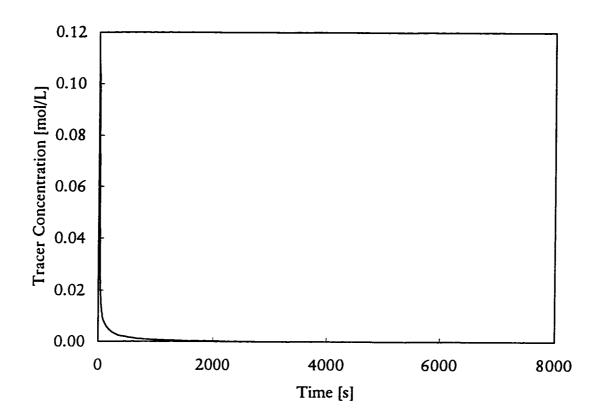
Figure S.1 Typical concentration vs. time profile from a tracer experiment; liquid flow rate: 480 mL/min
