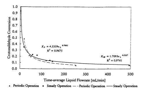
Figure 4.39 Steady and periodic operation (20 min period, 0.5 split) crotonaldehyde conversion vs. liquid flow rate, 50°C, 0.1 MPa
