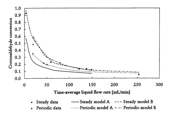
Figure 7.26 Comparison of periodic and steady operation model with experimental data at 50°C and 0.1 MPa; periodic operation parameters: 0.5 split 20 minute period
