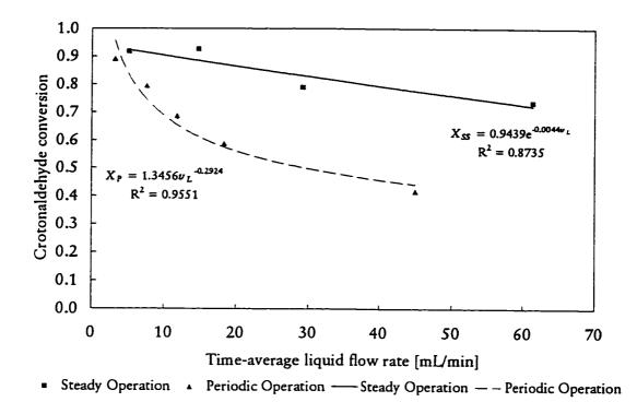
Figure 4.26 Steady and periodic operation 5 min period, 0.1 split Crotonaldehyde conversion vs. Liquid flow rate, 50°C, 1.1 MPa
