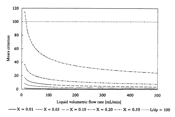
Figure 2.3 Mears Criterion for Neglecting Axial Dispersion as a Function of Conversion and Liquid Volumetric Flow rate for the Experimental Trickle-bed  $(L/d_p)$  is the ratio of catalyst bed length to catalyst particle diameter)
