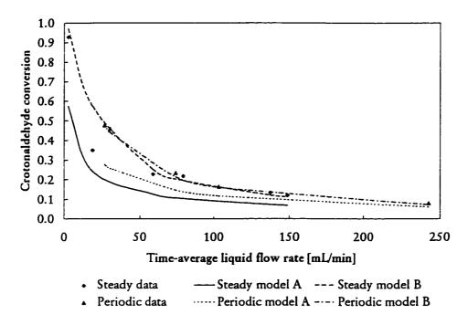
Figure 7.24 Comparison of periodic and steady operation model with experimental data at 50°C and 0.1 MPa; periodic operation parameters: 0.5 split 5 minute period
