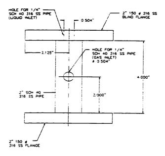
Figure 3.4 Inlet section
