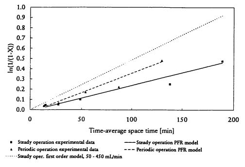
Figure 4.22 Steady and periodic operation (20 min period, 0.1 split), first order rate law plot, 25 °C, 1.1 MPa, liquid flow rate range: 0 - 50 mL/min
