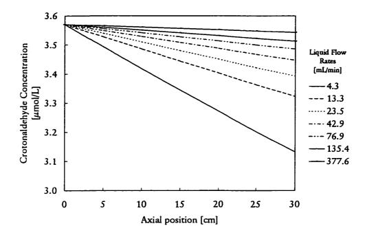
Figure 7.7 Bulk liquid phase crotonaldehyde concentrations as predicted by simulation Model A under steady operation at 25°C and 1.1 MPa
