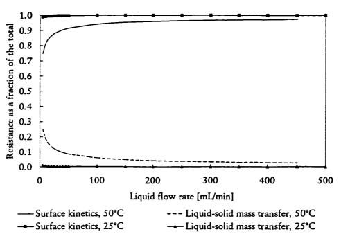
Figure 4.7 Contributing resistances to overall reaction rate as a function of liquid flow rate for steady operation at 25°C and 50 °C, 1.1 MPa, assuming a liquid-solid mass transfer coefficient twice that predicted by the Goto-Smith correlation
