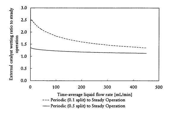
Figure 4.19 Ratio of external catalyst wetting under periodic operation (5 minute period) to that under steady operation as a function of time-average liquid flow rate
