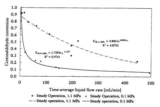
Figure 4.32 Steady operation crotonaldehyde conversion vs. liquid flow rate, 50°C, 0.1 MPa and 50°C, 1.1 MPa
