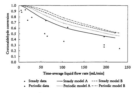
Figure 7.18 Comparison of periodic and steady operation model with experimental data at 50°C and 1.1 MPa; periodic operation parameters: 0.5 split 5 minute period
