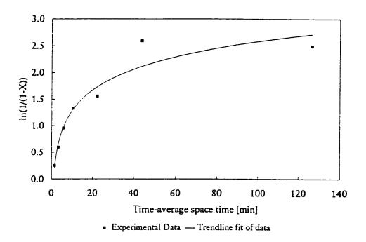
Figure 4.25 Steady operation first order plot, 50°C, 1.1 MPa
