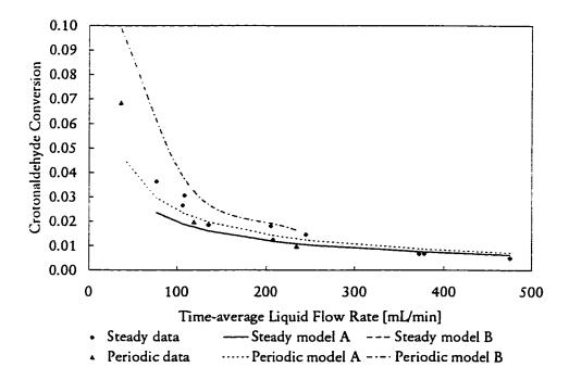
Figure 7.10 Comparison of periodic and steady operation model with experimental data at 25 °C and 1.1 MPa; periodic operation parameters: 0.5 split 5 minute period
