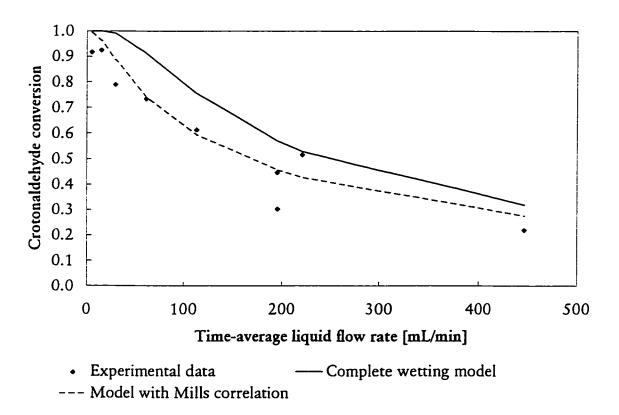
Figure 7.13 Steady operation Model A assuming variable catalyst external wetting with experimental data (Mills-Dudukovic wetting correlation used) and complete catalyst wetting (f = 1)
