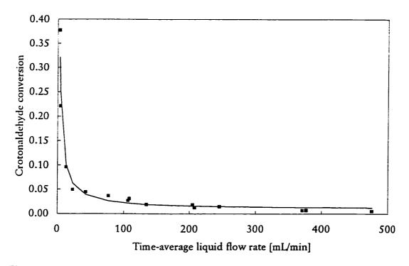
Figure 4.9 Crotonaldehyde conversion vs. liquid flow rate under steady operation, 25 °C, 1.1 MPa, liquid flow rate range: 0 to 450 mL/min
