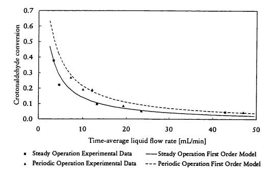
Figure 4.17 Steady and periodic operation (5 min period, 0.1 split), 25 °C, 1.1 MPa, Conversion vs. Liquid flow rate
