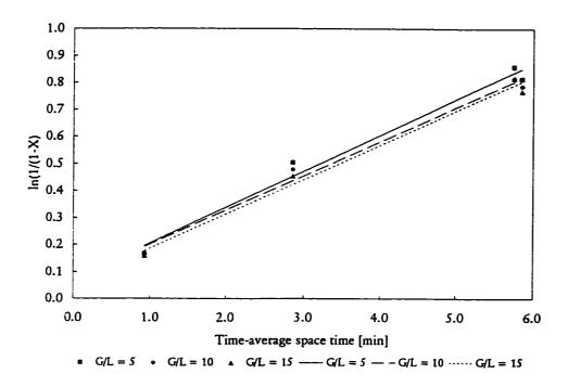
Figure 6.2 First order plot of steady operation data at different gas/liquid ratios
