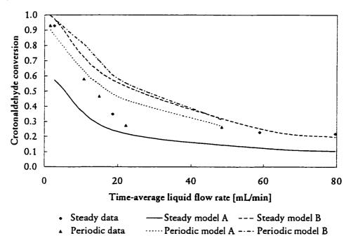
Figure 7.23 Comparison of periodic and steady operation model with experimental data at 50°C and 0.1 MPa; periodic operation parameters: 0.1 split 5 minute period
