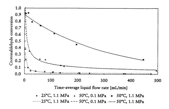
Figure 4.4 Steady-state crotonaldehyde conversion vs. liquid flow rate data for 25°C, 1.1 MPa, 50°C, 1.1 MPa, and 50°C, 0.1 MPa
