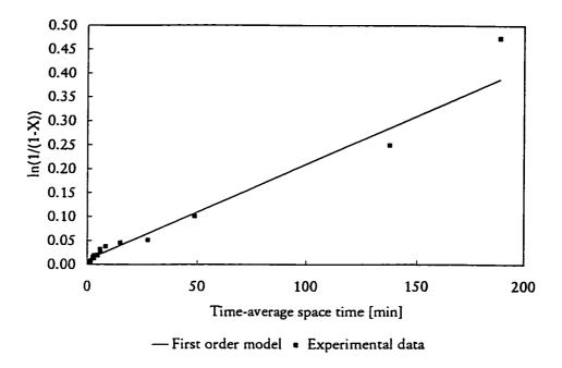
Figure 4.10 First order rate law plot for steady operation, 25 °C, 1.1 MPa, liquid flow rate range: 0 - 450 mL/min
