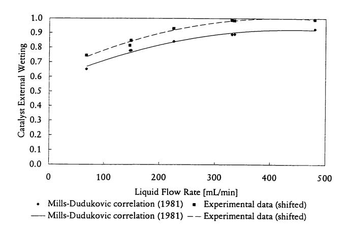
Figure 5.5 Catalyst external wetting as a function of liquid flow rate with experimental data shifted
