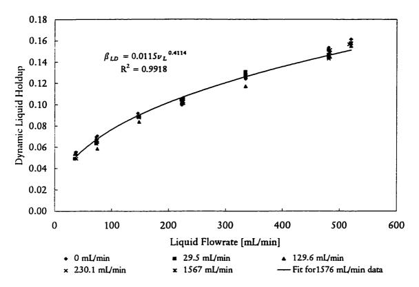
Figure 5.3 Dynamic liquid holdup as a function of liquid and gas flow rate
