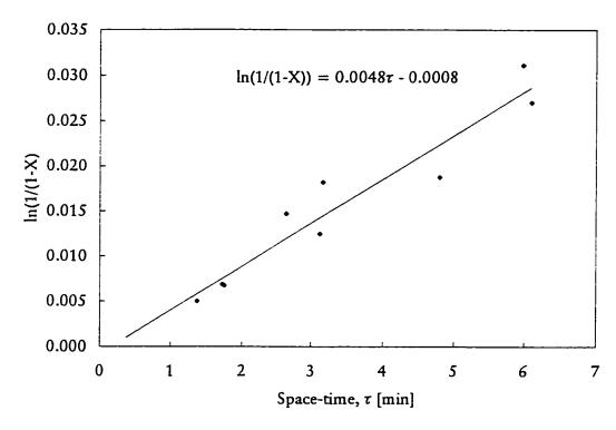
Figure 4.2 First order plot of steady-state data at high liquid flow rates (greater than 100 mL/min) for 25°C and 1.1 MPa
