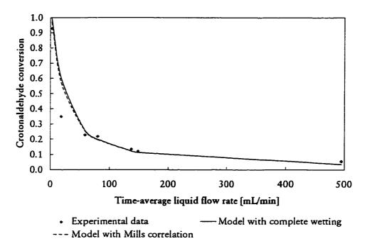
Figure 7.22 Steady operation Model B assuming variable catalyst external wetting with experimental data (Mills-Dudukovic wetting correlation used) and complete catalyst wetting (f = 1)
