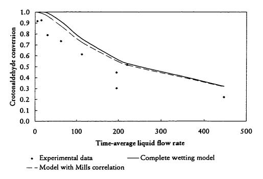
Figure 7.14 Steady operation Model B assuming variable catalyst external wetting with experimental data (Mills-Dudukovic wetting correlation used) and complete catalyst wetting (f = 1)
