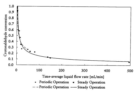
Figure 4.34 Steady and periodic operation (5 min period, 0.1 split) crotonaldehyde conversion vs. liquid flow rate, 50°C, 0.1 MPa
