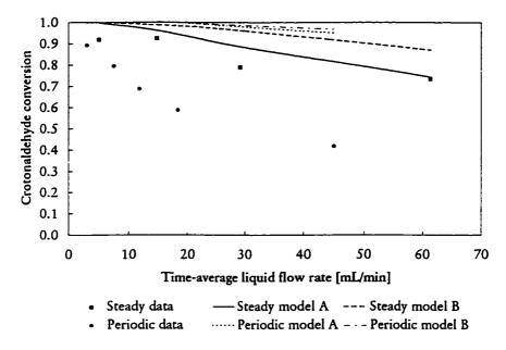
Figure 7.17 Comparison of periodic and steady operation model with experimental data at 50°C and 1.1 MPa; periodic operation parameters: 0.1 split 5 minute period
