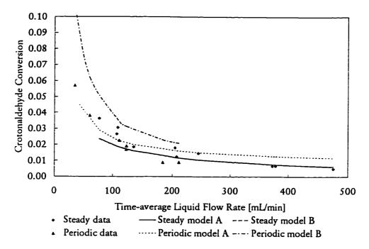
Figure 7.12 Comparison of periodic and steady operation model with experimental data at 25 °C and 1.1 MPa; periodic operation parameters: 0.5 split 20 minute period
