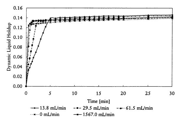
Figure 5.2 Time response of dynamic liquid holdup drainage from the catalyst bed as a function of gas flow rate
