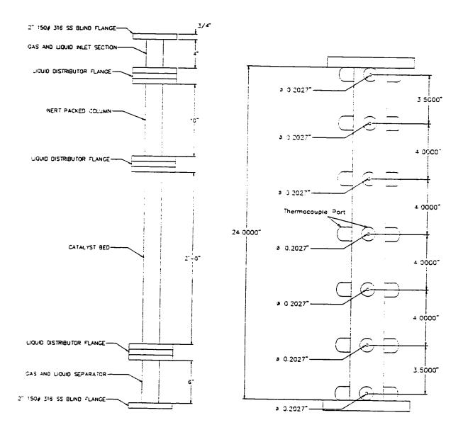
Figure 3.2 Trickle-bed reactor
