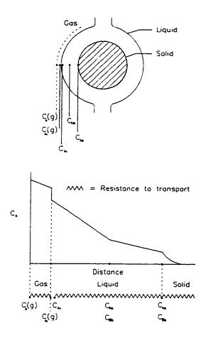
Figure 2.1 Concentration profiles for trickle-bed reactors (Fogler 1986)
