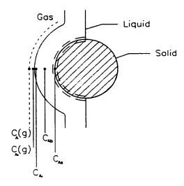
Figure 7.1 Gas-liquid-solid contact at the particle level for Model A
