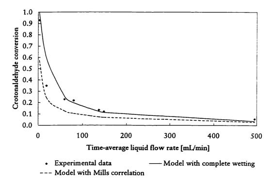
Figure 7.21 Steady operation Model A assuming variable catalyst external wetting with experimental data (Mills-Dudukovic wetting correlation used) and complete catalyst wetting (f = 1)
