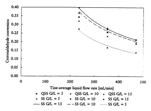
Figure 6.7 Comparison of Quasi-Steady and Periodic Operation Crotonaldehyde Conversion - Effect of Flush Duration
