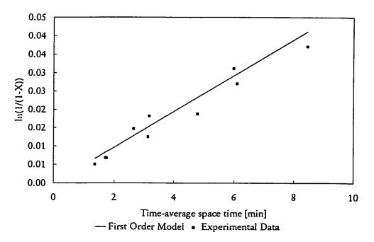
Figure 4.13 Steady operation first order plug flow model, 25°C, 1.1 MPa, liquid flow rate range: 50 - 450 mL/min
