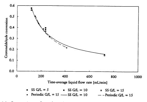
Figure 6.3 Comparison of steady and periodic operation crotonaldehyde conversion - effect of cycle period
