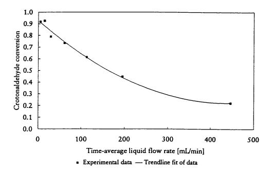
Figure 4.24 Steady operation crotonaldehyde conversion vs. liquid flow rate, 50°C, 1.1 MPa
