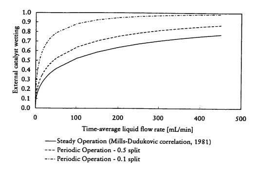
Figure 4.18 Comparison of catalyst external wetting under steady and periodic operation as a function of time-average liquid flow rate
