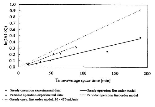
Figure 4.16 Steady and periodic operation (5 min period, 0.1 split) first order rate law plot, 25 °C, 1.1 MPa, liquid flow rate range: 0 - 50 mL/min
