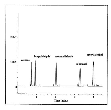
Figure M.1 Sample Gas Chromatograph
