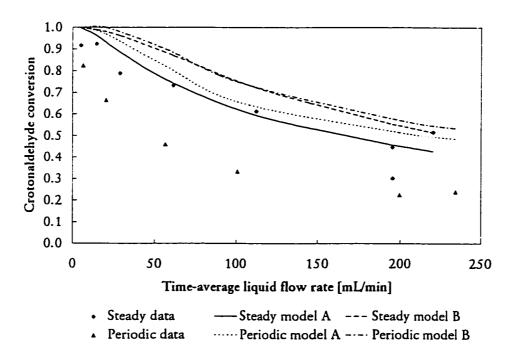
Figure 7.20 Comparison of periodic and steady operation model with experimental data at 50°C and 1.1 MPa; periodic operation parameters: 0.5 split 20 minute period
