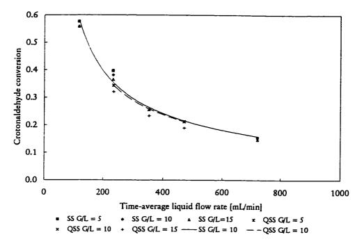
Figure 6.5 Comparison of quasi-steady and steady crotonaldehyde conversion
