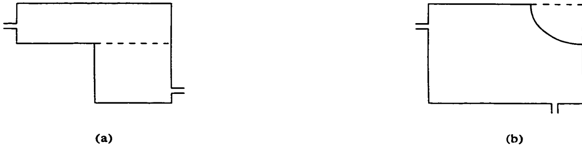
Figure 2.2: (a) Planar circuit, composite of two canonical shapes, can be analyzed by segmentation method (b) Non-canonical planar circuit which will have a canonical shape by adding a canonical shape, can be analyzed by desegmentation method.
