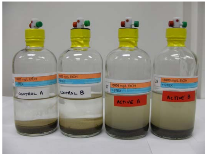
Figure 2.5 Photograph of microcosms from treatment series G (15000 mg/L ethanol + BTEX) at the end of the experiment (Day 67). Note the cloudy grey appearance of the liquid phase and the black precipitate in the aquifer material of active microcosms.
