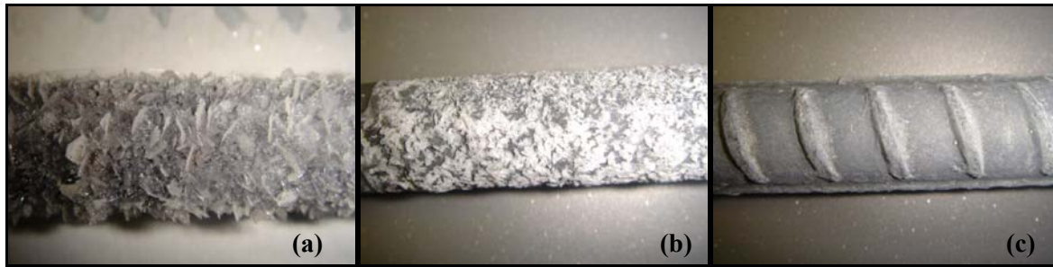
Figure 4-8. CHZ formed on bars with different coatings in pH 13.7 (a) non-chromated, (b) annealed, and (c) chromated
