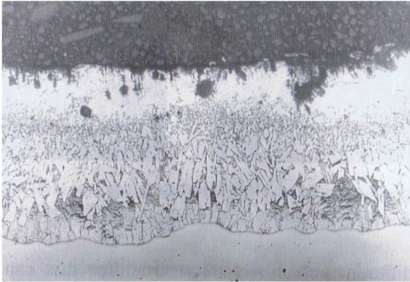
Figure 2-10. Dissolution of pure zinc surface layer during passivation [7]
