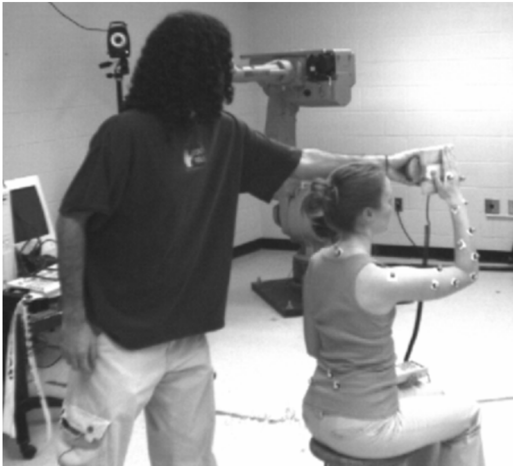
Figure 7: Photo of experimental trial. Subject is horizontally adducting against force transducer held by experimenter. Digital display in left hand was used to help maintain constant force. Direction of force was assumed to be perpendicular to the palm of the hand.
