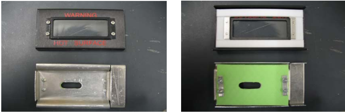
Figure 3-6: Original and customized environmental chamber cover.
