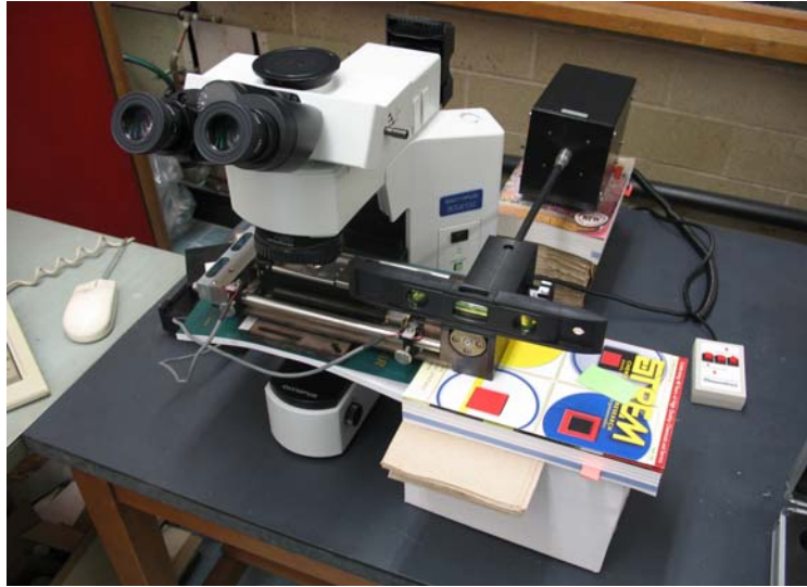
Figure 3-4: Apparatus set up with Minimat underneath the microscope.
