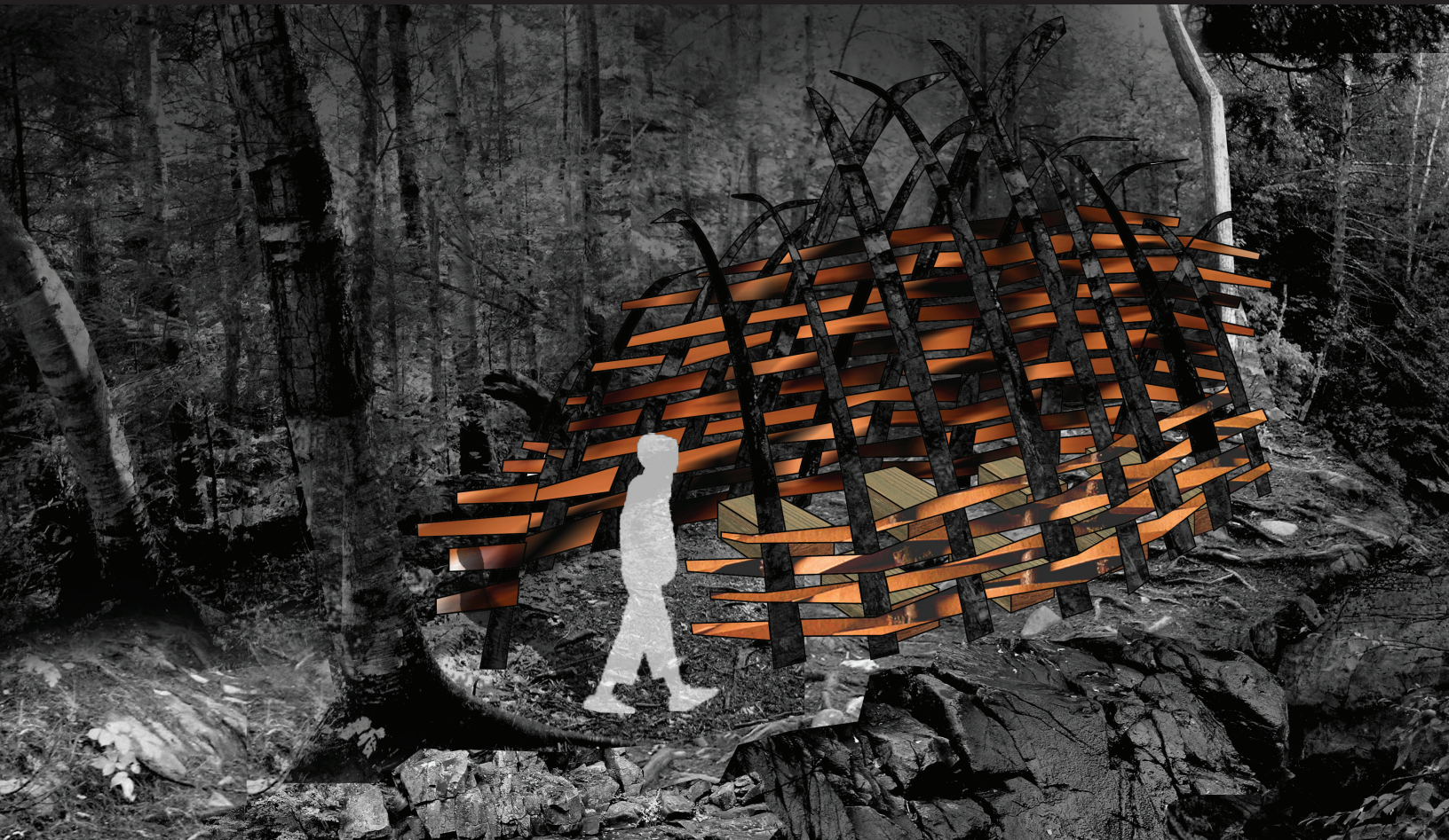
9.16 Chapel overlooking Ragged Falls, made of timber members and interlaced with copper strips.
