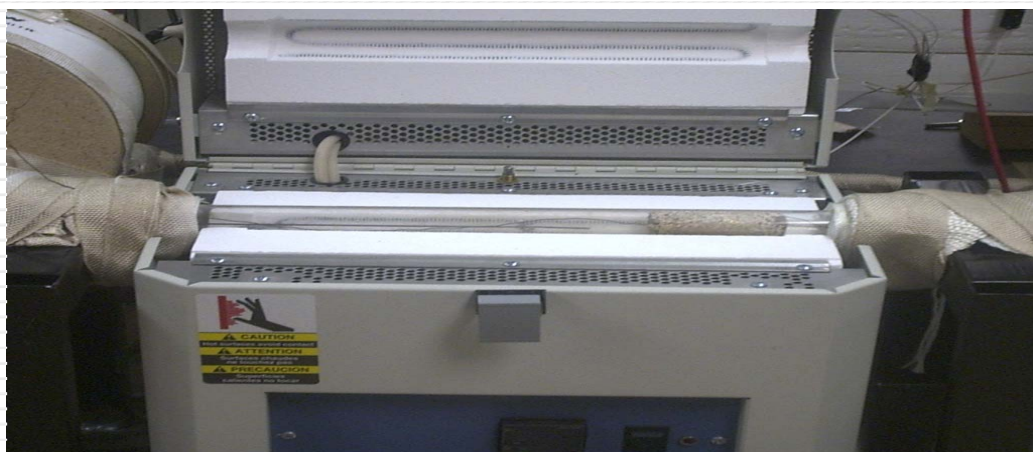
Figure 3-1 Reactor and catalyst section
