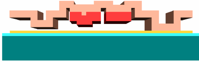
Figure 5-30: CoventorWare TM simulation of three gaps which can be fabricated with PolyMUMPs.
