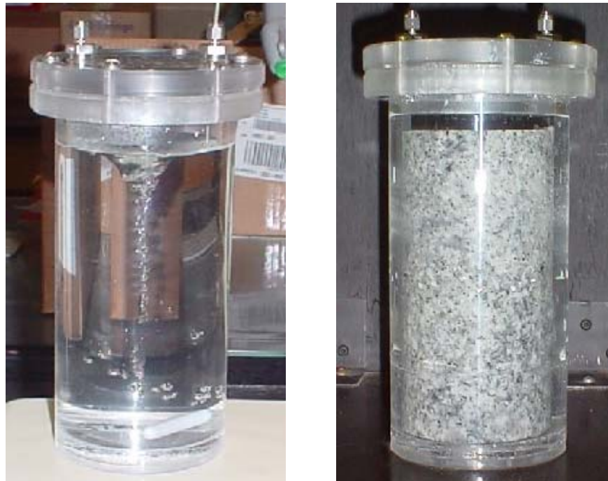
Figure 5. Experimental Set-up for the Out-diffusion Experiment
