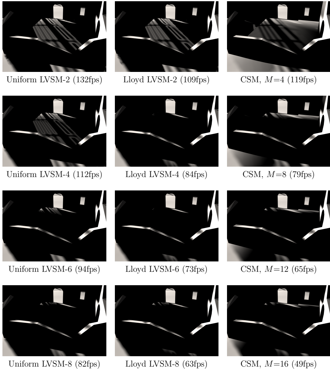
Figure 4.5: Comparison between convolution shadow maps and layered variance shadow maps. LVSM- N indicates LVSM with N layers. Each row of the grid uses an equal amount of storage. Performance numbers were taken at 1920 \times 1200 , 4 \times MSAA with a 1024 \times 1024 shadow map.
