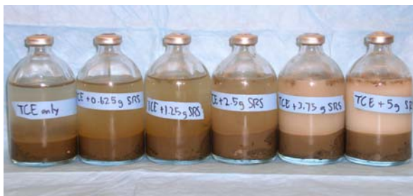
Figure 4.4 SRS TM Partitioning Experiment Reactor Bottles
