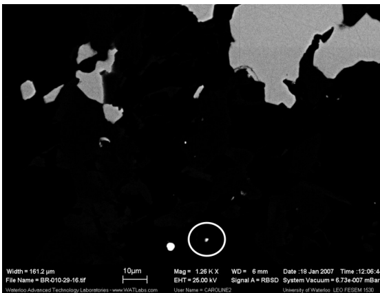
39: PGM – Froodite ( \text{PdBi}_2 ) grain within silicate gangue groundmass.
