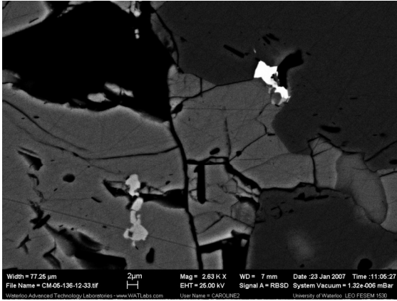
3: PGM - Merenskyite ( \text{PdTe}_2 ) at the pentlandite and serpentine grain boundary.
