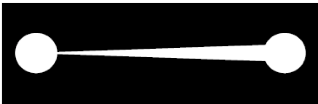
Figure 15: Design 2 (dimension 60 \mu\text{m} height, 400 \mu\text{m} narrow end and 4000 \mu\text{m} wide end)
