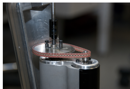
Figure 2.16: APK servomotor powered gearing
