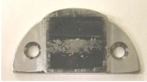
Figure 2.5: CNTs were peeled off at very high bias and deposited on the anode.
