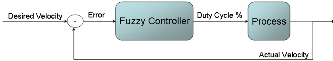
Figure 3.5: Block diagram of the error-based fuzzy controller.
