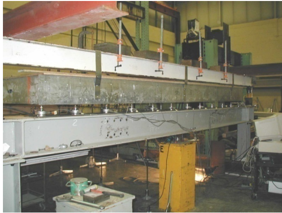
Figure 3.22: Load Sharing Test
