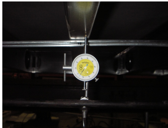
Figure 3.20: Dial Gauge Setup for Deflection Test
