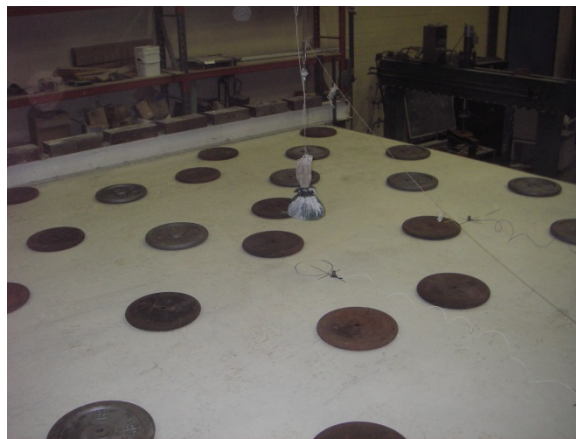
Figure 4.3: Live Load Applied to Laboratory Floor System
