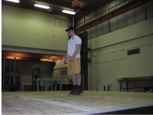
Figure 3.13: Heel Drop Test
