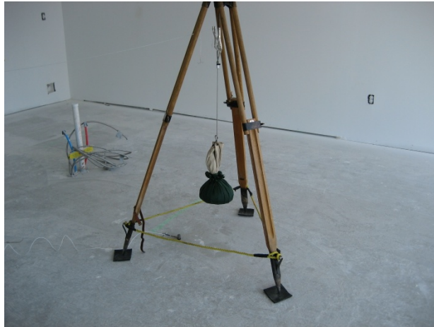
Figure 3.17: Sandbag Test as Performed in the Field
