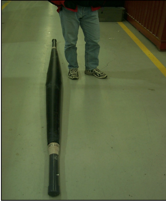
Figure A-23: Tapered FLUTE Packer- Deflated (left), Inflated (right)
