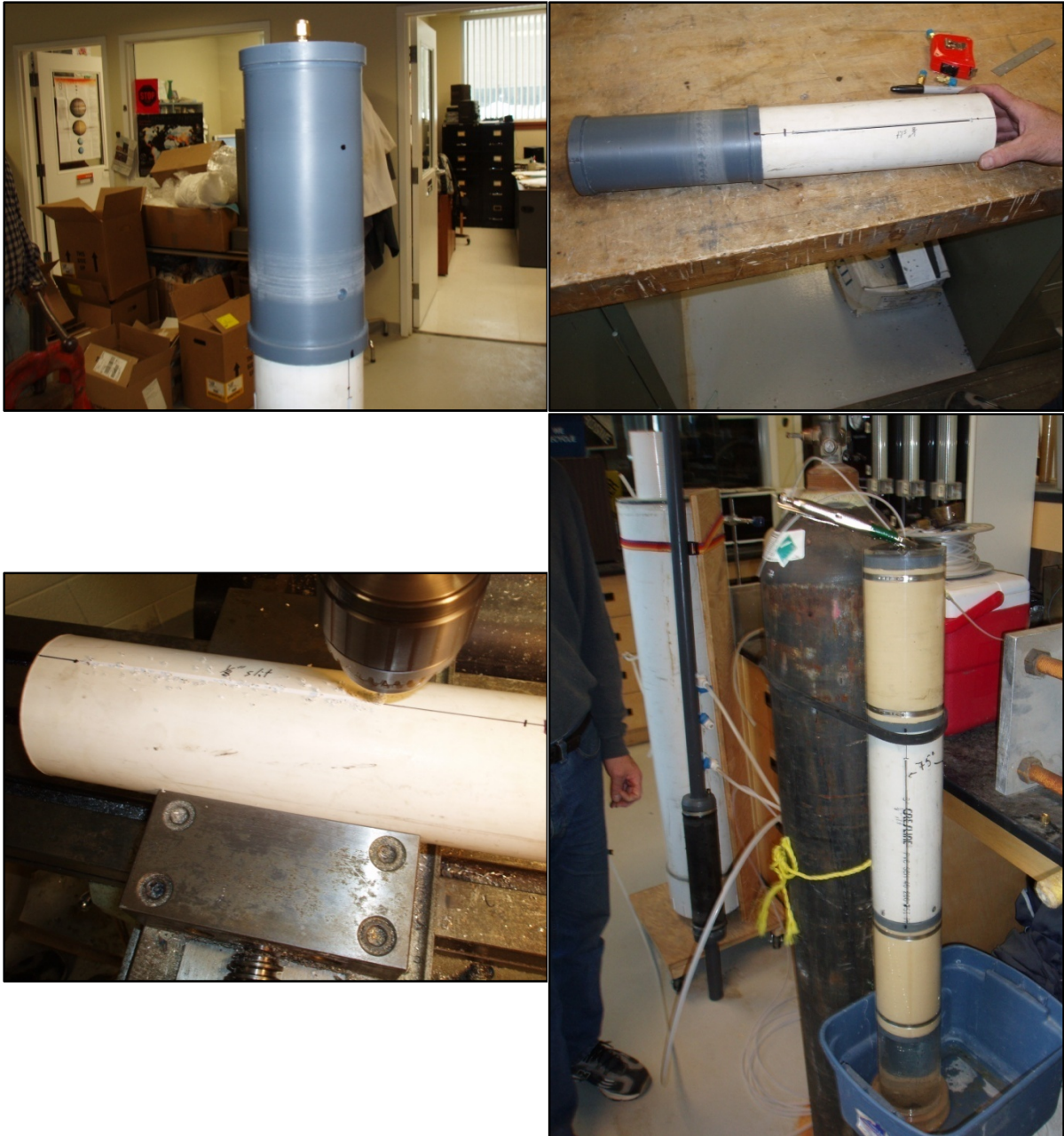
Figure A-25: Vertical Slit Straddle Packer Design and assembly process. Vertical slit is spaced 75 degrees apart, and is 12" long set between two packers.
