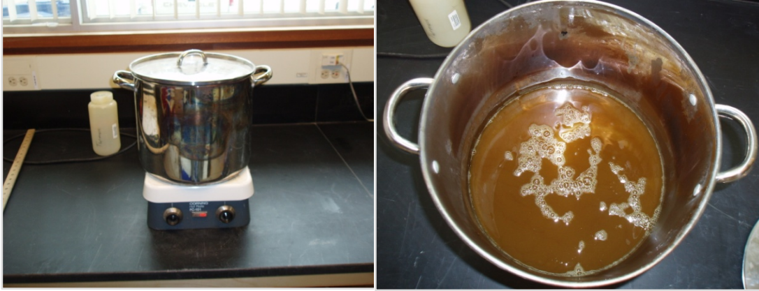
Figure 2-11: Dyeing Set-up, 9L pot on hot plate used to simmer material for 1hr.
