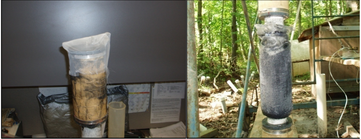
Figure A-13: Assembly issues with Straddle Packer GAC design, issues with putting sock on, and sloughing of GAC
