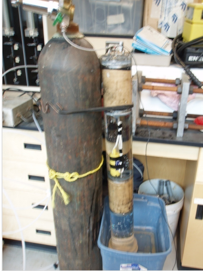
Figure 2-4: Plexi-glass well used to examine prototype. This well gave the ability to see leaks in a packer, the mixing disturbance created with different volts sent to the mixing pump (used for borehole dilution tests). This is a no flow system, and used strictly as a visual indicator of what happens in a borehole.
