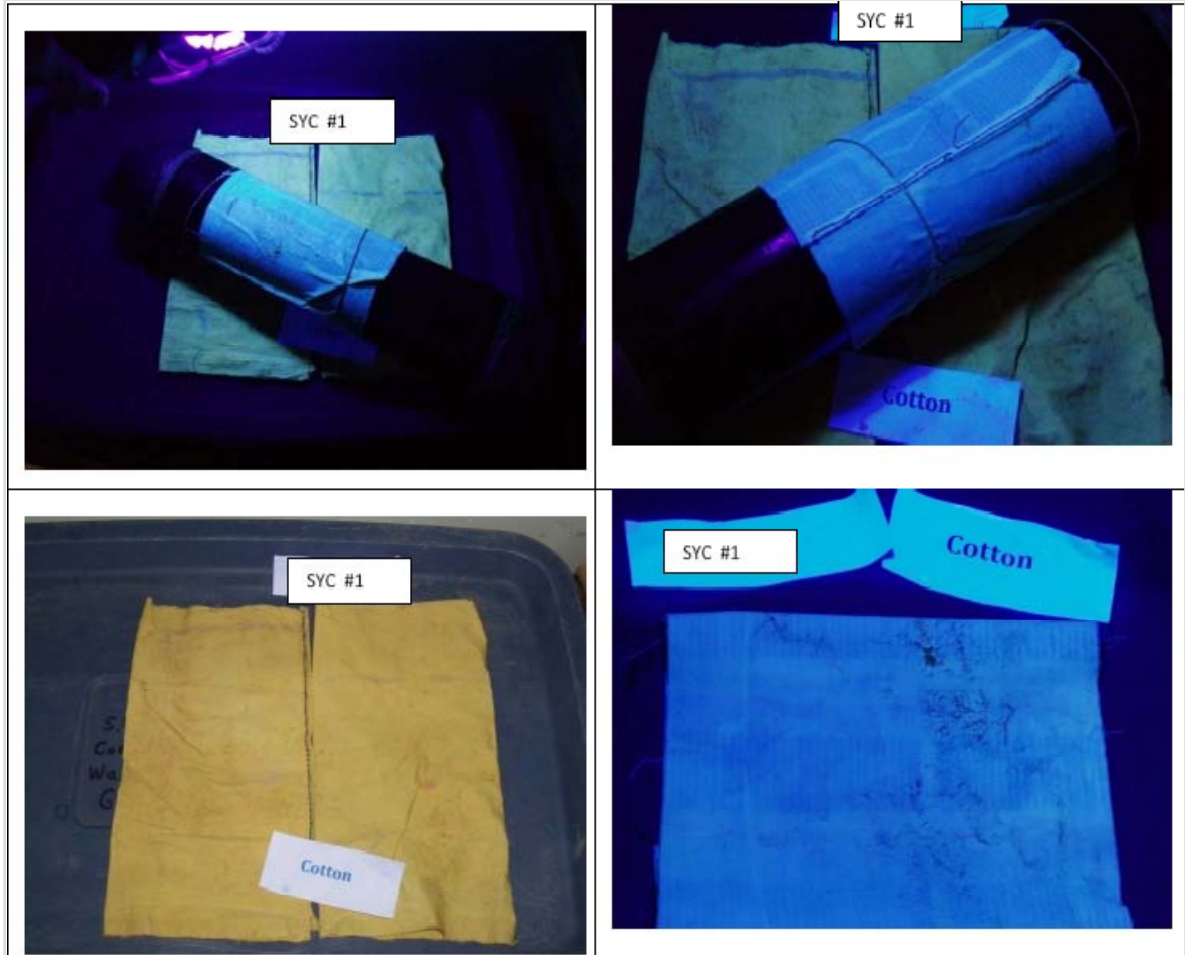
Figure 3-14: Steeping Test - top left shows the result after six hours steeping; top right shows the result five days after steeping; bottom left shows the dry normal results after five days; bottom right shows the dry black light results after five days steeping. The packer and material was placed in the laboratory well and left to soak for five days to see how much influence flow actually had on the colour change that occurs. As shown, the colour change is not a vibrant, these show up very faint, as compared to when there are flow conditions.
