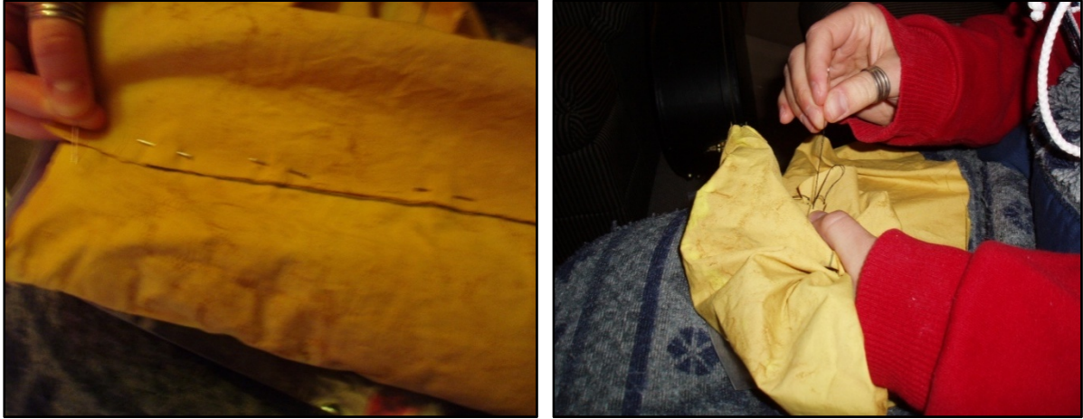
Figure 3-4: Sewing of Cotton/SYC #1 Sleeve. Cut to size, strips are dyed then hand sewn to fit on the packer. The fabric is sewn so the material fits tight on the packer, and thus needs to stretch with the packer when inflated.
