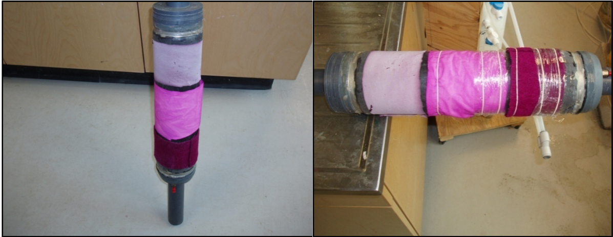
Figure 3-5: Dyed Test Strips on Packer. They are able to stay on the packer without aid. From bottom to top they are wool/AR52, cotton/AR52 and lycra/grape juice (Left). Elastics are used to ensure the material stays in place (Right), and the saran wrap is used to create a no-flow zone to see how the dyes react to porous media flow through a well screen.
