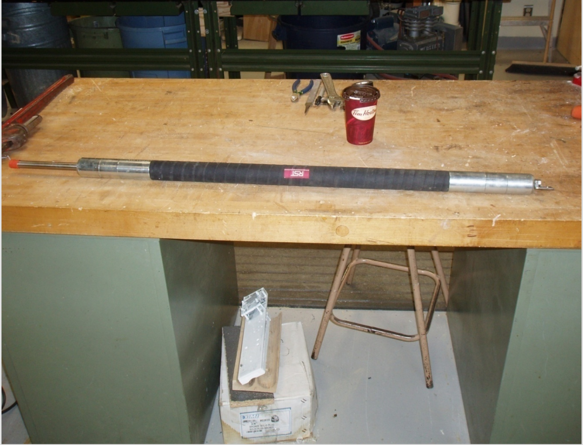
Figure 2-21: Standard Packer deflated
