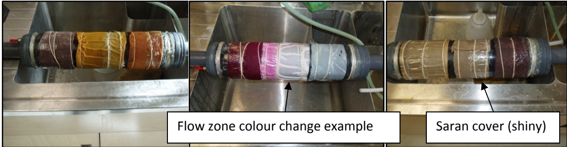
Figure 3-6: Strips on packer after it is removed from the box aquifer. Notice the colour changes between the zones that had flow and those with no flow. The flow zone was created by wrapping part of the material with Saran wrap, this is impermeable so flow could not affect this zone. The elastics moved but the material stayed in place. From left to right: wool/blueberries, cotton/SYC #1, wool/SYC #1, wool/AR52, cotton/AR52, lycra/blueberries, cotton/tea, lycra/tea, wool/grape juice.
