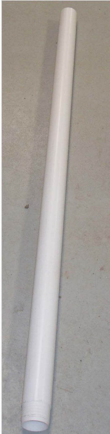
Figure 2-7: Images of well screen slits. The left image is a full length 10 slot (0.01inch, 0.245mm) well screen. Each well slot is 254 \mu m in this 10cm diameter well screen. The two images on the right show a close-up of these slots. Notice the inside slots are shorter than the outside, this is due to the curvature of the well screen and how the knife cuts through the well.
