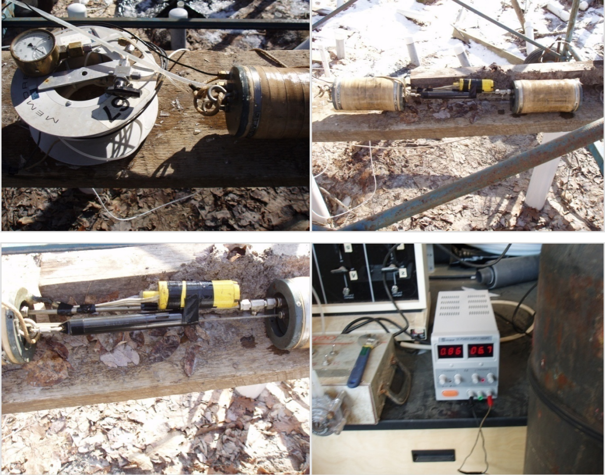
Figure A-16: Borehole Dilution Set-up - Inflation Line, Whale Pump, CTD Diver and Power supply
