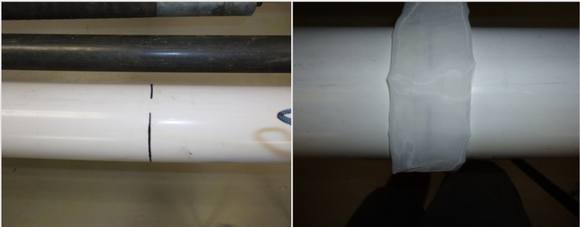
Figure 2-8: Simulated Fracture Slit (4.78mm) (Left) Simulated Fracture covered with Nytex (Right)
