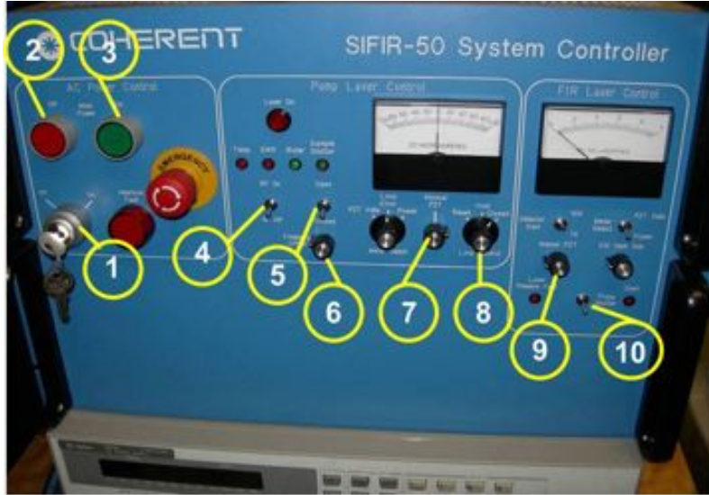
Figure 2.5: Front panel of the SIFIR-FPL system controller. Some main components: main power key (1), green on button (2), red off button (3), pump laser RF ON switch (4), frequency offset knob (6), pump PZT (7), loop control knob (8), FIR PZT (9), pump shutter(10) [Captured by author in Terahertz Research Center, RPI]
