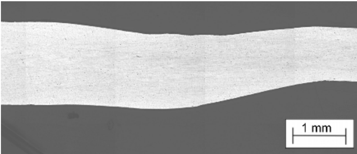
Figure 4.57: Low aspect ratio weld specimen produced with a welding power of 1.8 kW at a welding speed of 20 mm/s showing that the weld is free of solidification micro-porosity.
