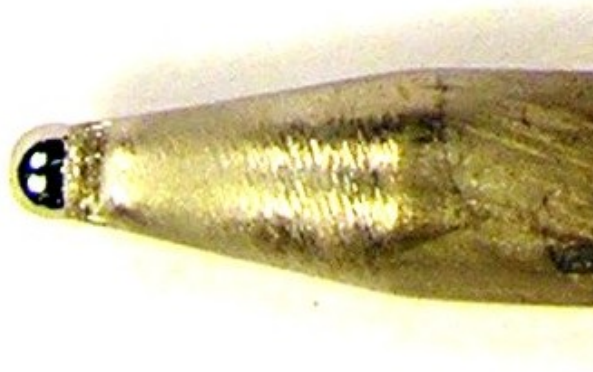
Figure 4.11: Image of a ground 4.8 mm diameter electrode after welding showing the shape of the molten balled tip formed during welding.
