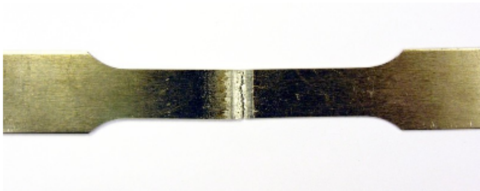
Figure 4.42: Typical transverse tensile specimen failure.
