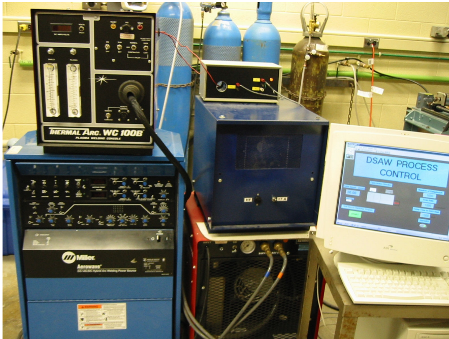
Figure 3.1: DSAW welding system including: power supply, plasma console, pilot arc booster, water recirculator and data acquisition and control system (taken from Kwon [29].)
