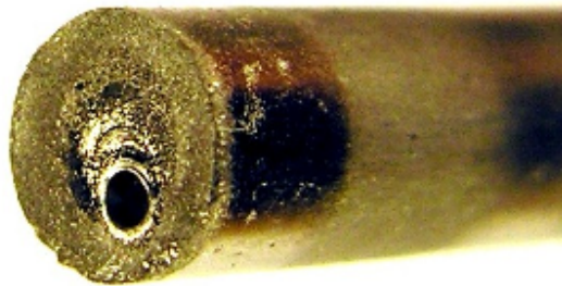
Figure 4.12: Images of a blunt 4.8 mm diameter electrode after welding showing little evidence of significant melting of the electrode tip during welding.
