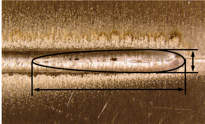
Figure 4.55: Weld pool crater at the end of the PAW side of specimen showing the length and width measurements used to determine the aspect ratio of the weld pool.
