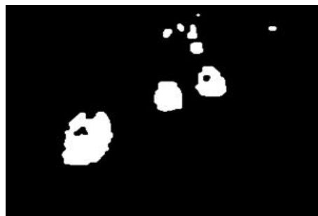
Figure 6.21: GMM result of Gaussian added noise image after morphological post-processing and image filtration with Wiener filter.
