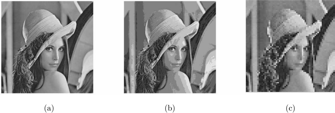
Figure 9.2: (a) Original, Grey-levels: 8 bits, Size: 512 by 512, (b) Low brightness resolution, Grey-levels: 3 bits, Size: 512 by 512, (c) Low spatial resolution, Grey-levels: 8 bits, Size: 64 by 64 (replicated for larger view).
