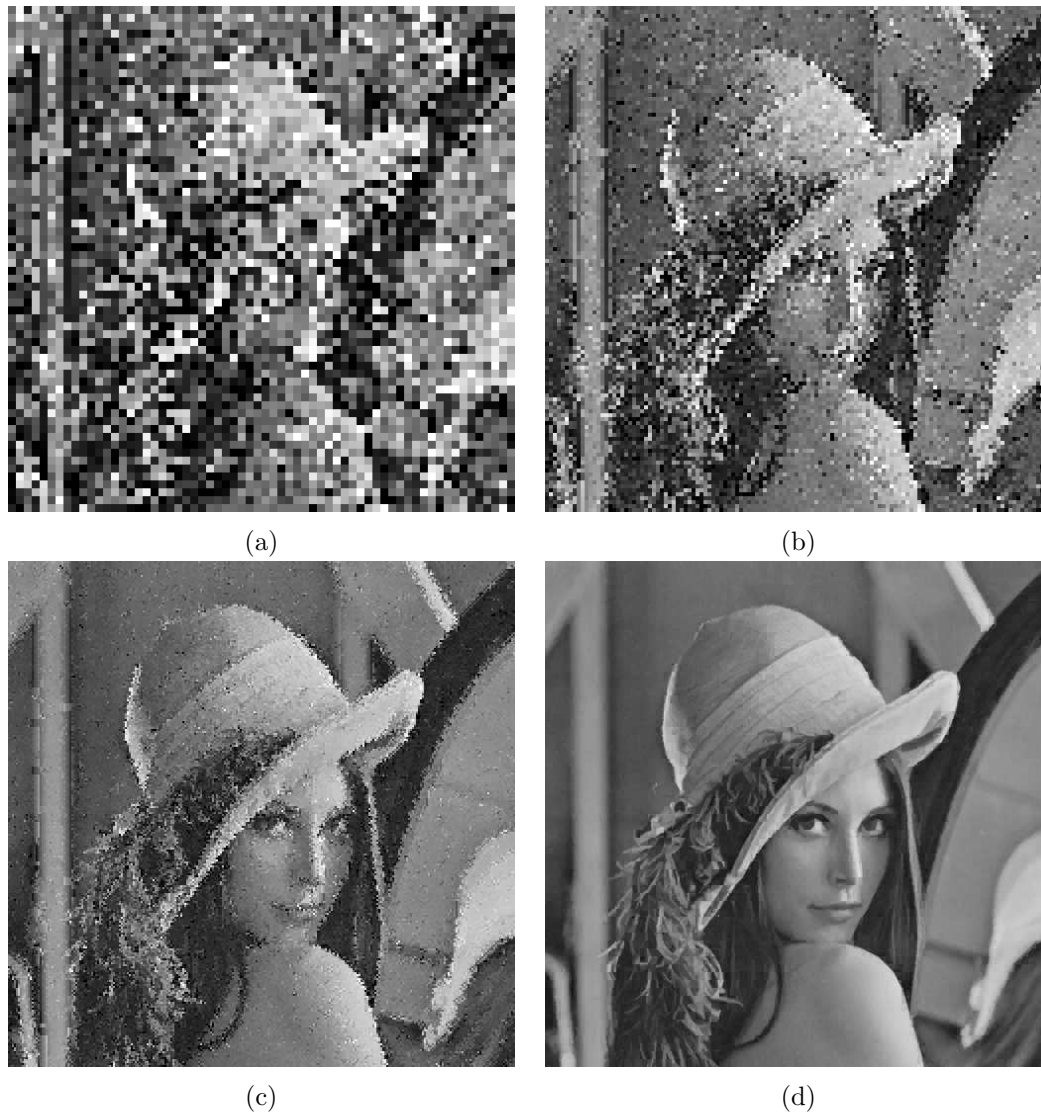
Figure 3.5: The iterates \mathbf{u}_1 , \mathbf{u}_2 and \mathbf{u}_3 , are respectively plotted in (a), (b), and (c). The fixed point \mathbf{u}^* of the fractal transform operator T designed to approximate the standard 512 \times 512 (8 bpp) “Lena” image is shown in (d). The “seed” image was \mathbf{u}_0(x, y) = 255 (plain white). The fractal transform T was obtained by “fractal coding” using 4096 nonoverlapping 8 \times 8 pixel range blocks. The domain pool consisted of the set of 1024 nonoverlapping 16 \times 16 pixel blocks.
