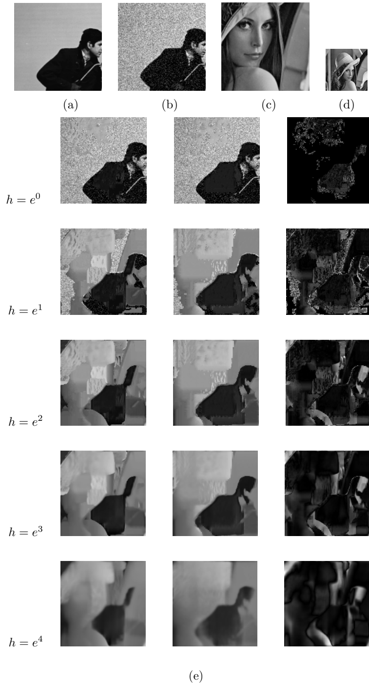
Figure 8.9: (a) shows the original image \mathbf{x} , (b) the observation \mathbf{u} , (c) \mathbf{v}_1 , (d) \mathbf{v}_2 = \mathcal{D}_2(\mathbf{v}_1) , (e) For each value of h , Left hand-side: \tilde{\mathbf{x}}_{(\mathbf{u}, \mathbf{v}_1, h, d, a)}(x) , middle: \tilde{\mathbf{x}}_{(\mathbf{u}, \mathbf{v}_2, h, d, a)}(x) , right hand-side: |\tilde{\mathbf{x}}_{(\mathbf{u}, \mathbf{v}_1, h, d, a)}(x) - \tilde{\mathbf{x}}_{(\mathbf{u}, \mathbf{v}_2, h, d, a)}(x)| .
