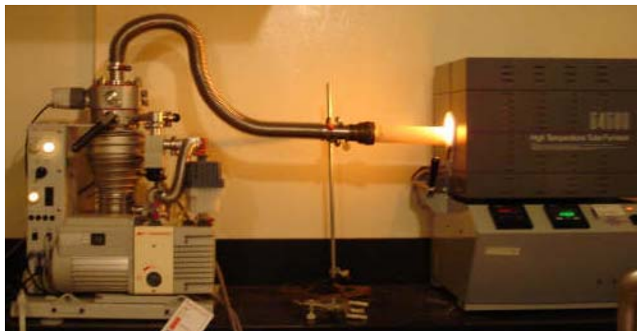
Figure 2.3 High temperature furnace with the Diffstak Mk2 diffusion oil pump.
