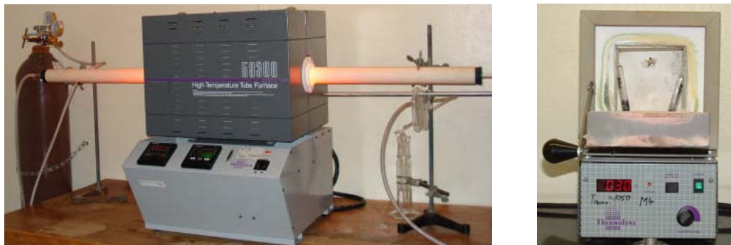
Figure 2.2 Tube furnace (left); box furnace with the gas flow (right).
