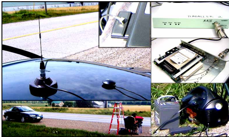
Figure 3.2: Equipment: Soekris board (top right), 802.11 PCMCIA card in laptop with external antenna connector (middle top), Magnetic 7 dBi Antenna and Magnetic USB GPS Receiver (left), Vehicle and roadside access point (laptop with antenna on ladder) (bottom left), and the two power units used to power the access point (bottom right).
