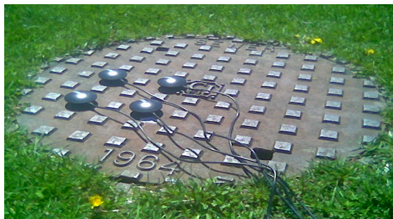
Figure 3.3: Arrangement of GPS devices used for Stationary Measurements.
