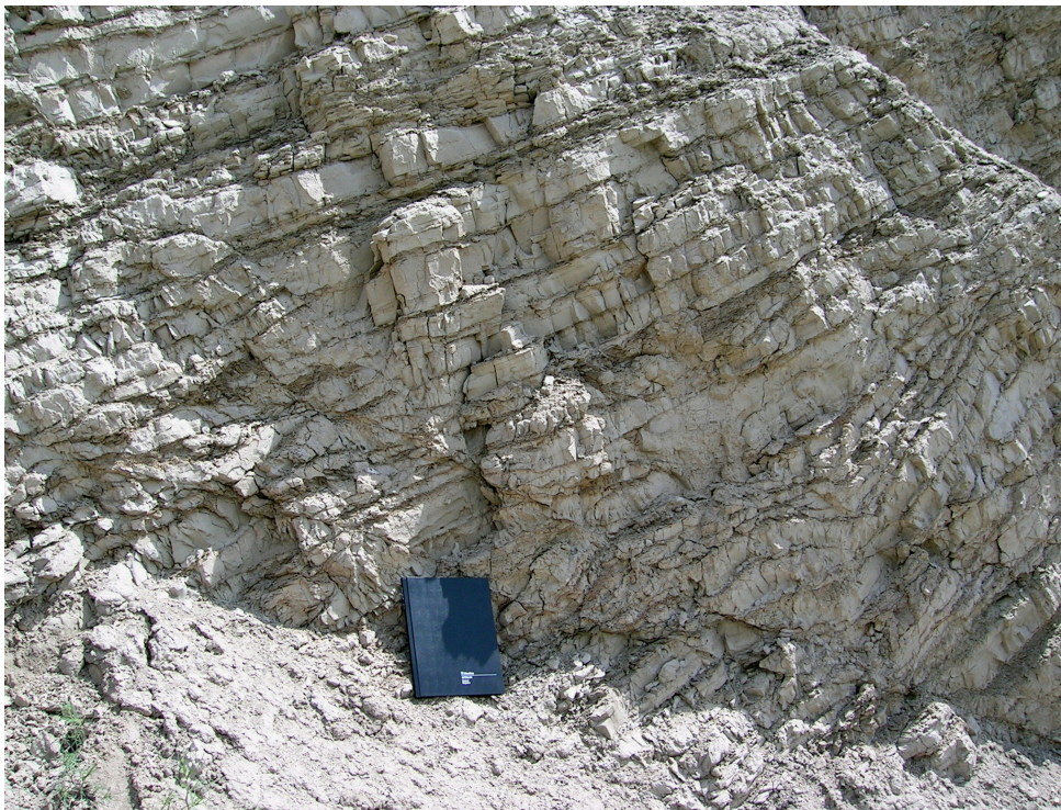
Figure 2 - 3. Photographs of undisturbed interbedded silt and clay (above), and disturbed silt and clay (below), Thompson River Valley, near Ashcroft, British Columbia. Dark layers are clay interbeds, and light layers are silt interbeds. Note the stratigraphic sections are dominated by silt interbeds.
