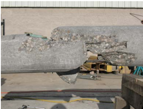
c) Failed section (loading side)
