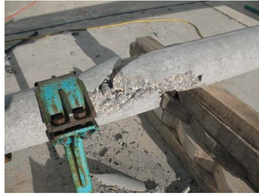
b) Failure at collar (loading side)
