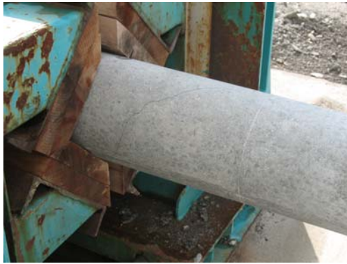
a) Initial cracking at butt
