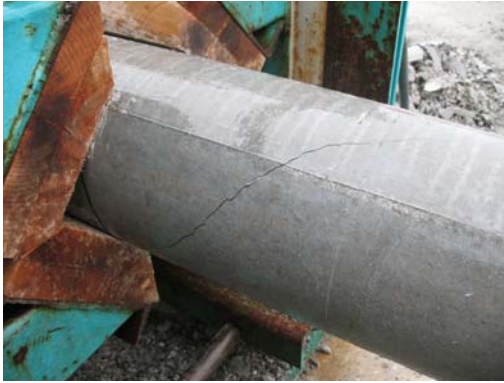
a) Initial cracking at butt
