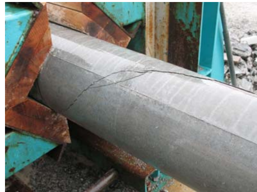
d) Cracks at butt after failure at collar
