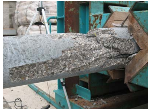
f) Failed section (loading side)
