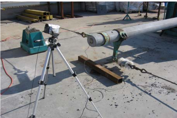
c) Loading and tie-back collar setup
