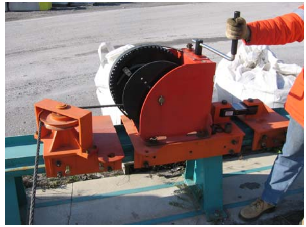
b) Application of loads using two-speed manual winch
