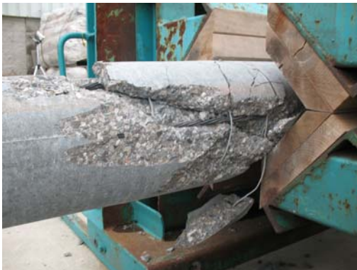
e) Failure at butt (loading side)
