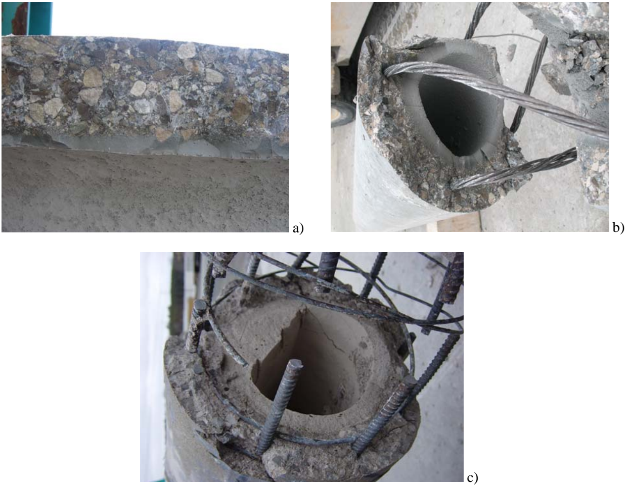
Figure 7.34 a)-c): a) Typical paste wedge and segregation along inner wall of specimens b) segregation of 210-CCW-L specimen c) extreme example from Chahrour and Soudki (2006) pole testing
