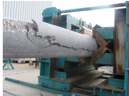
f) Crack pattern (loading side)
