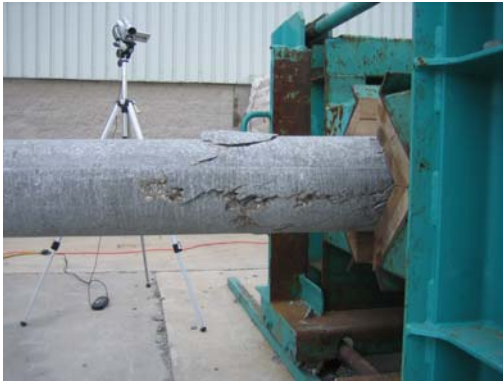
c) Failed section (loading side)
