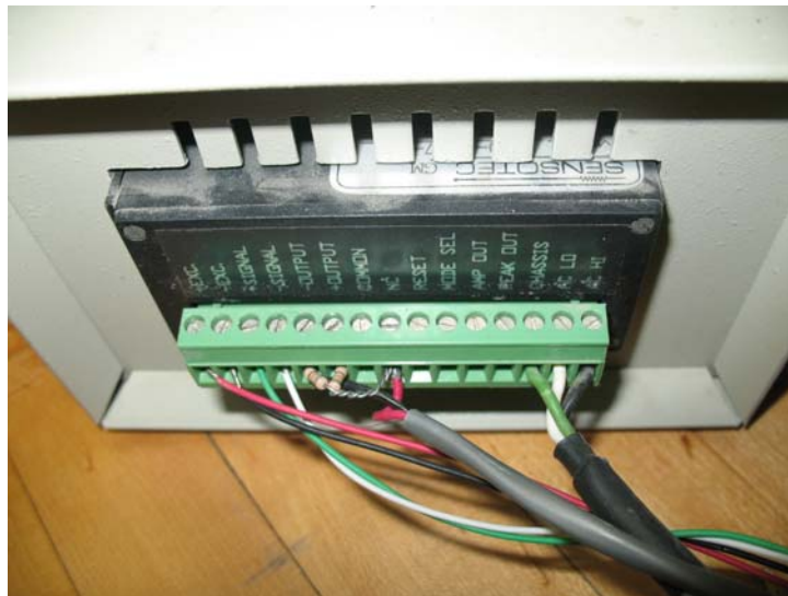
Figure 5.3: Signal conditioner with voltage divider
