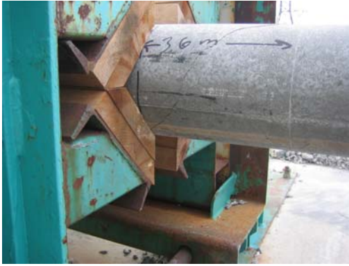
a) Initial torsional cracking at butt
