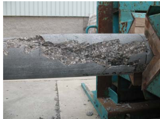
d) Failed section (loading side)
