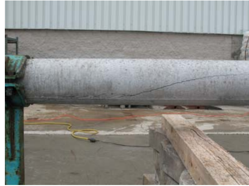
b) Torsional cracking prior to failure
