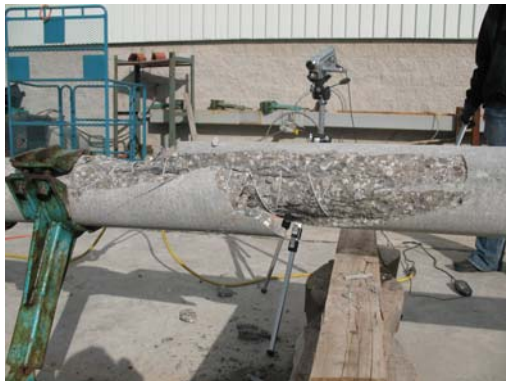
e) Failure at collar (loading side)
