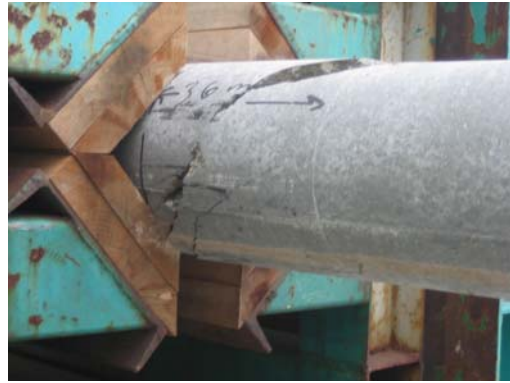
d) Failed section (back side)
