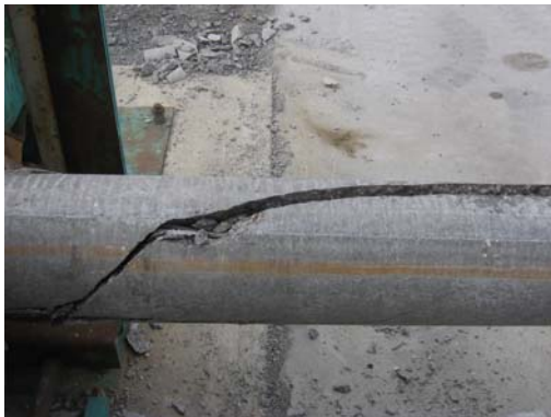
e) Crack pattern (back side)
