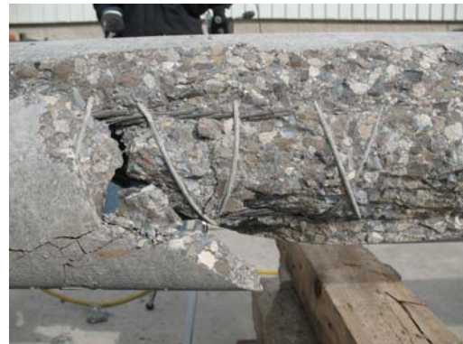
f) Double helix and confined concrete
