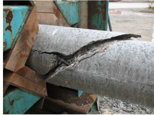
b) Failed section at butt (back side)
