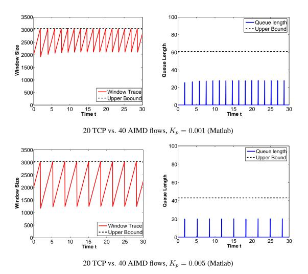
Figure 4.8: Bounds of Heterogeneous flows, C=60,000 packet/sec, R = 0.05 sec
