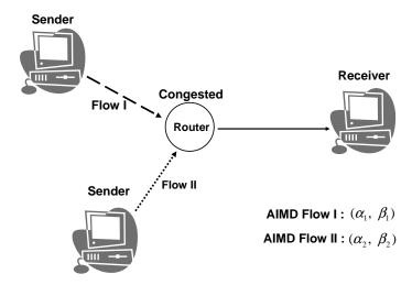
Figure 3.6: Heterogeneous AIMD/RED System
