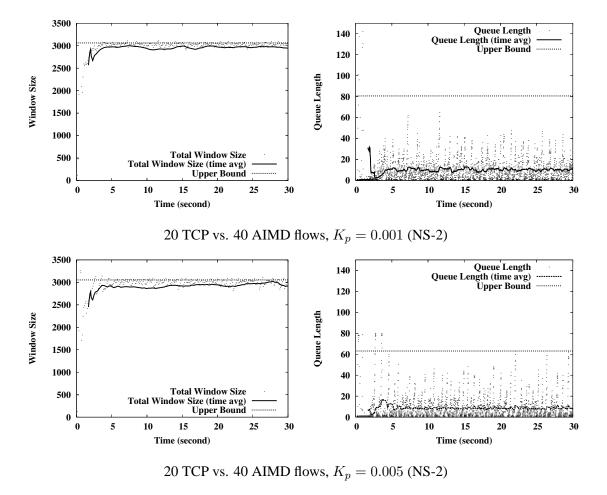
Figure 4.9: Bounds of Heterogeneous flows, C=60, 000 packet/sec, R = 0.05 sec
