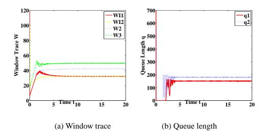
Figure 5.6: TCP and AIMD(0.2,0.875) flows, heterogeneous traffic in group I
