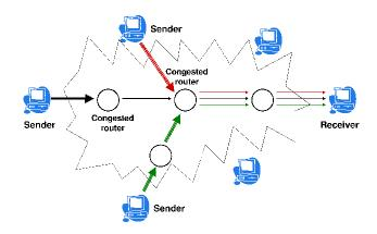
Figure 5.1: General Case of a Multiple-Bottleneck Network
