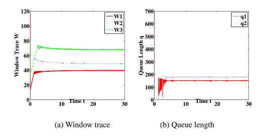
Figure 5.5: TCP and AIMD(0.2, 0.875) flows, delay-free
