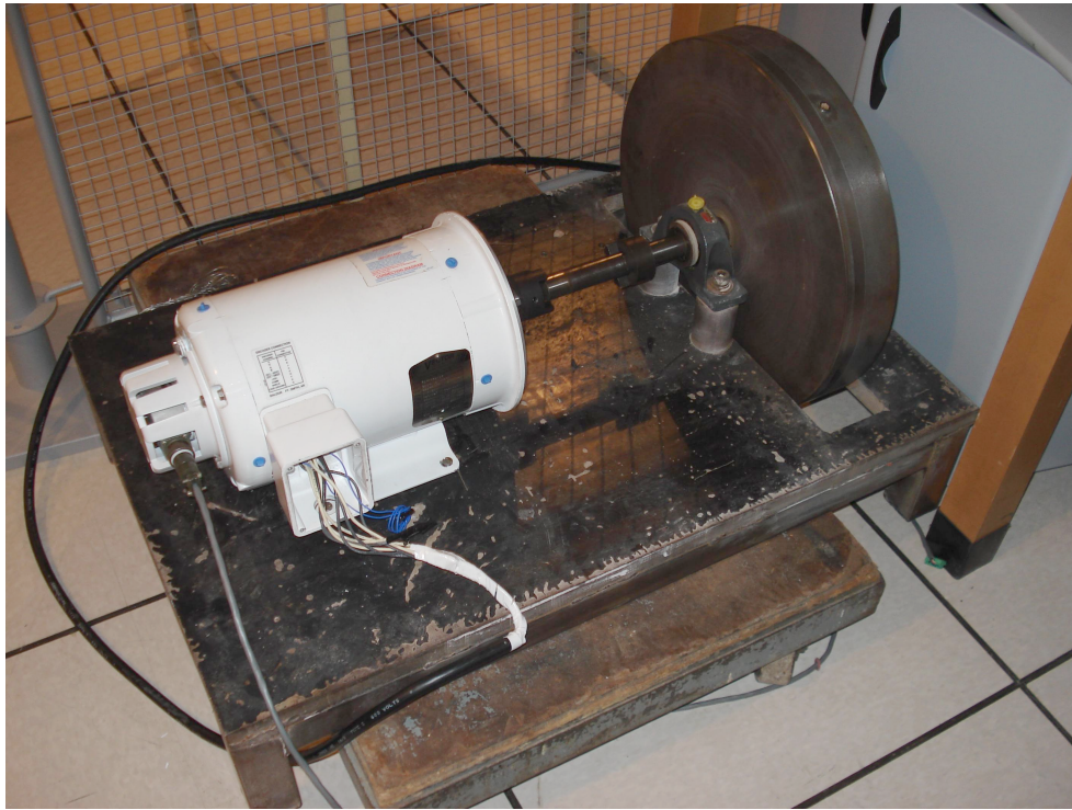
Figure 4.47: Original configuration of the testbench
