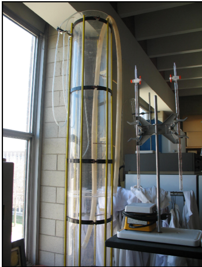
Figure 2.15: Example of a settling column for characterizing flocs.
