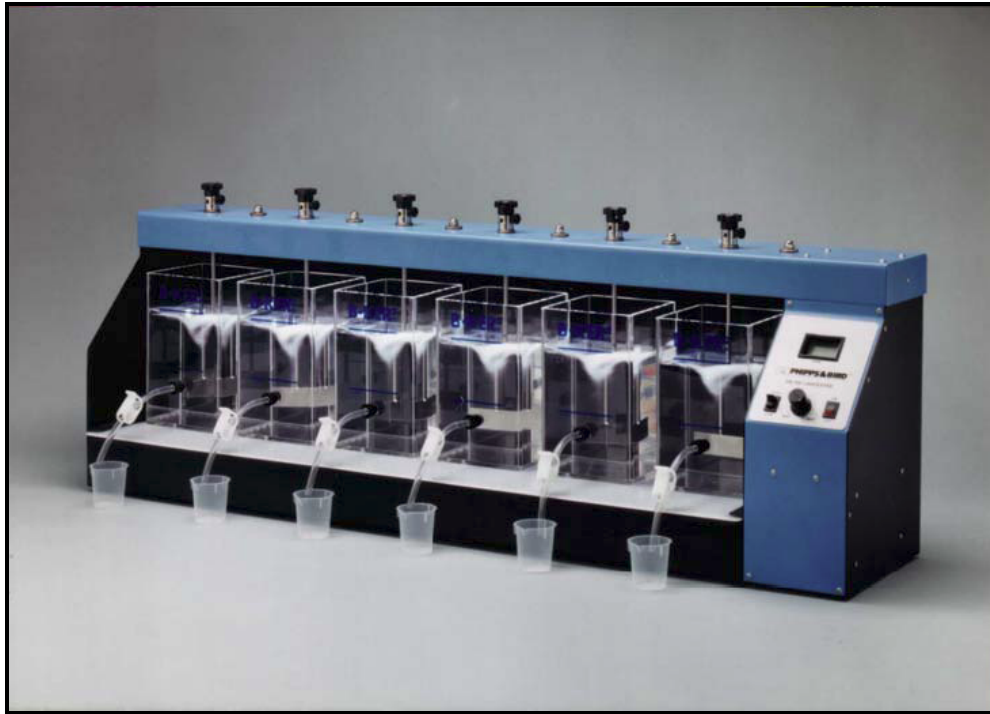
Figure 2.8: A Phipps & Bird standard jar tester (Grammer, 2007).
