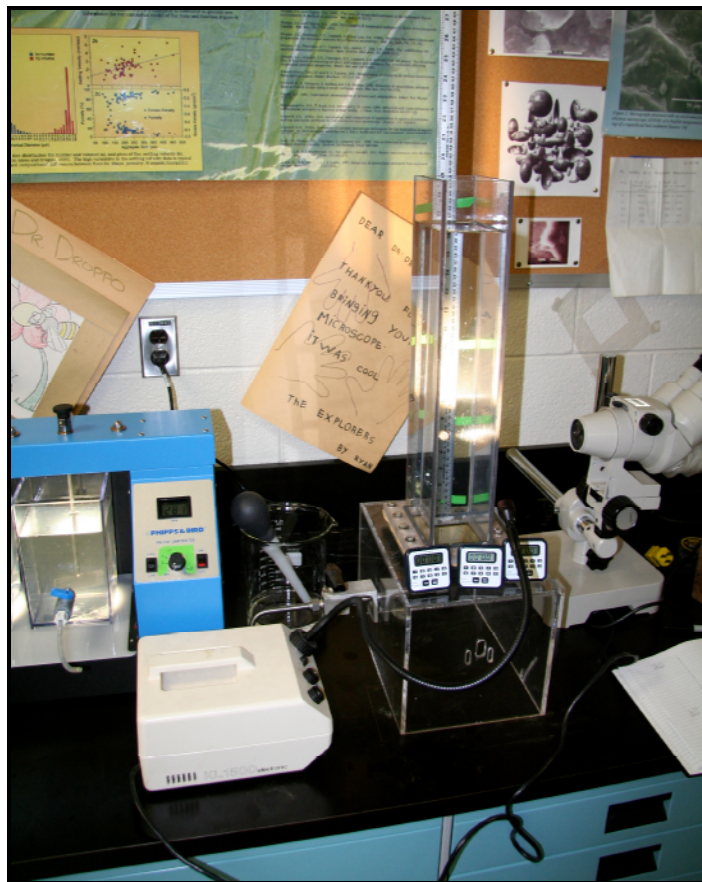
Figure 3.4: 2.5 L capacity settling column with a stereoscopic microscope.
