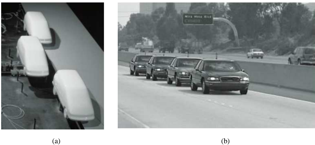
Figure 6.1: (a) Three-Lumina platoon in the Dryden wind tunnel at USC, and (b) platoon operation at 4-meter spacing to measure aerodynamic drag and fuel consumption [95].
