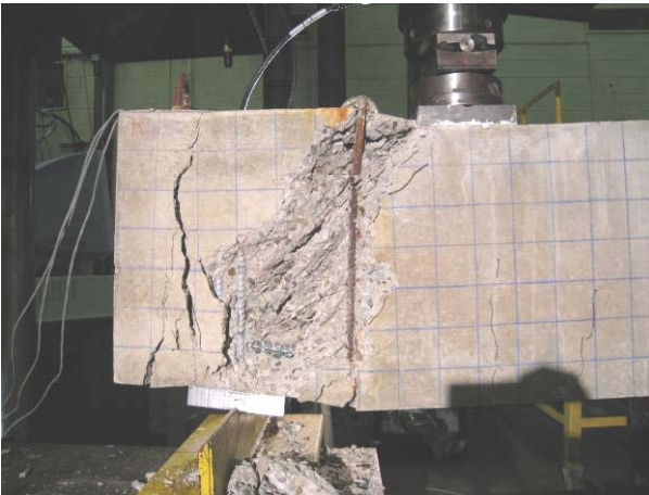
L-1.0-R (Diagonal Crushing)
