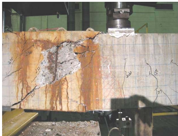
H(M)- 2.0-R (Diagonal Crushing)
