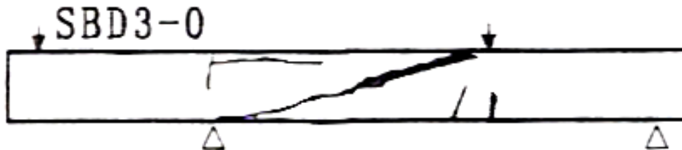
Figure 2.10 Beam Loading and Crack Pattern Kage et al. (1997)
