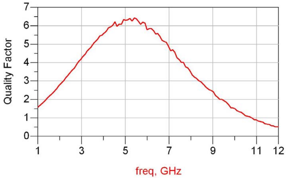
Figure 52: Measured Q of a fabricated RF MEMS tunable inductor based on an aluminum/PAA/aluminum sandwich structure at 0 V.
