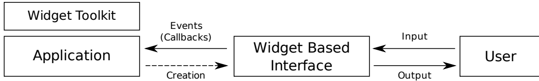
Figure 3.1: Model of widget toolkit based systems. Creation of the widget-based interface only happens once. User input and output is governed by the widget-based interface, which calls application code through an event system.
