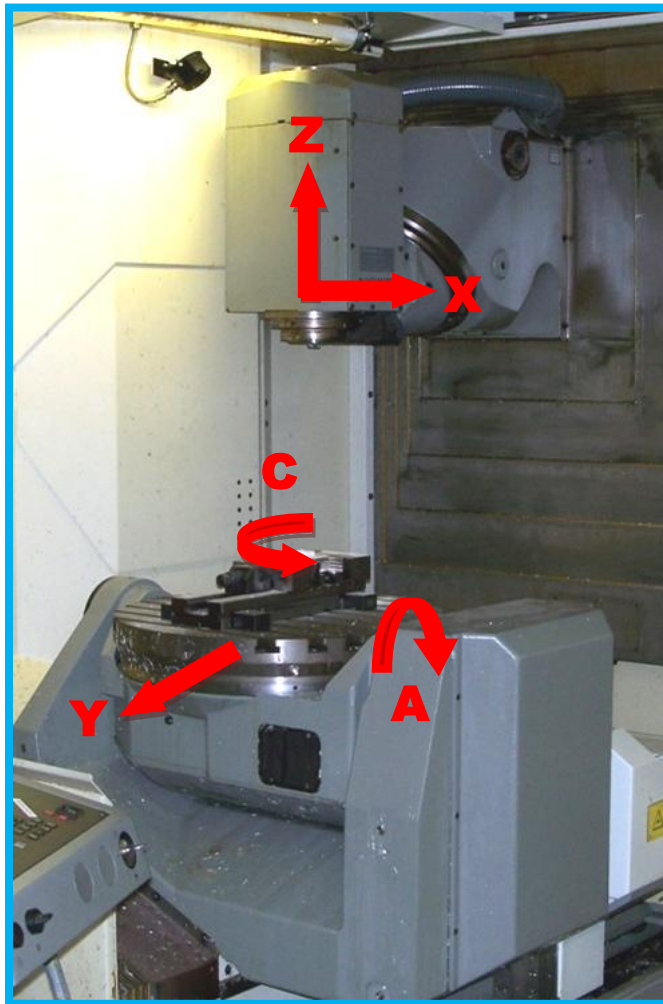
Figure 4-5: The DMG 80 P hi-dyn machine located at CIMLab with all 5 axis designated
