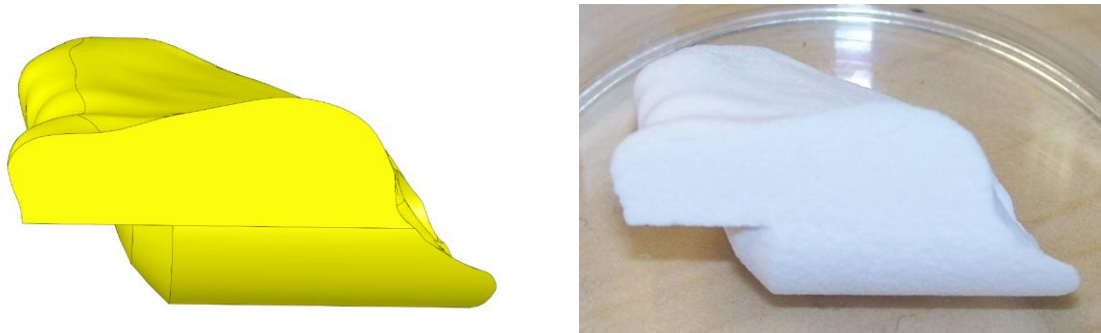
Figure 4-30: Final CPP Implant comparative figures from different angles, showing the CAD model on the left and the machined part on the right. Note that surface quality is acceptable and chipping is kept low and is not significant.
