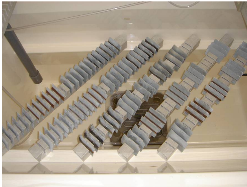
Figure 3-10: Placement of coupons on racks inside the corrosion chamber
