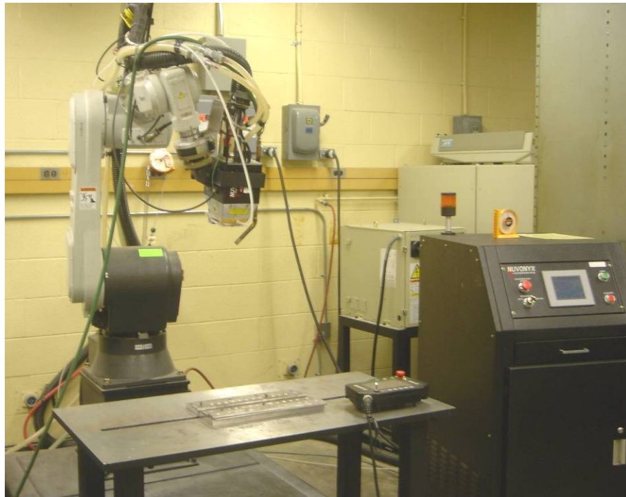
Figure 3-4: Welding setup of Nuvonyx diode laser on a robot
