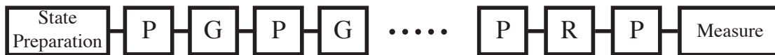
Figure 3.8: Quantum circuit implementing single qubit benchmarking. A fiducial state is prepared and a sequence of computational gates G is applied. The recovery gate R is chosen to return the state to fixed state. The Pauli gates P interleaved with the computational gates induce a Pauli randomization.
